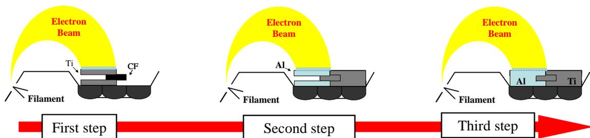
Fig. 4 Schematic diagram of preparation of Ti/Al junction with carbon fiber.
