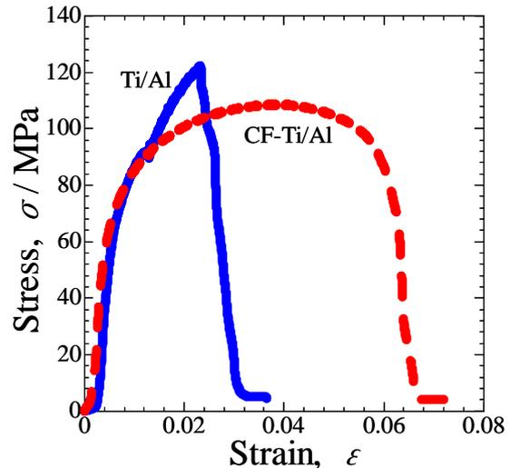
Fig. 9 Stress-strain curves of Ti/Al junctions with and without carbon fiber.
