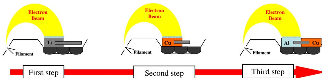
Fig. 3 Schematic diagram of preparation of Cu/Al junction with carbon fiber.
