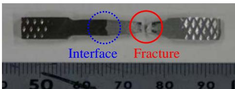
Fig. 8 Photograph of fractured sample of Ti/Al junctions with carbon fiber.
