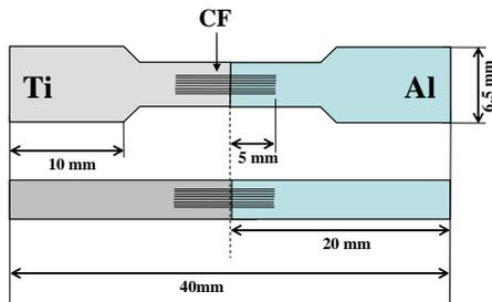
Fig. 7 Schematic diagram of joint sample of Ti/Al with carbon fiber.
