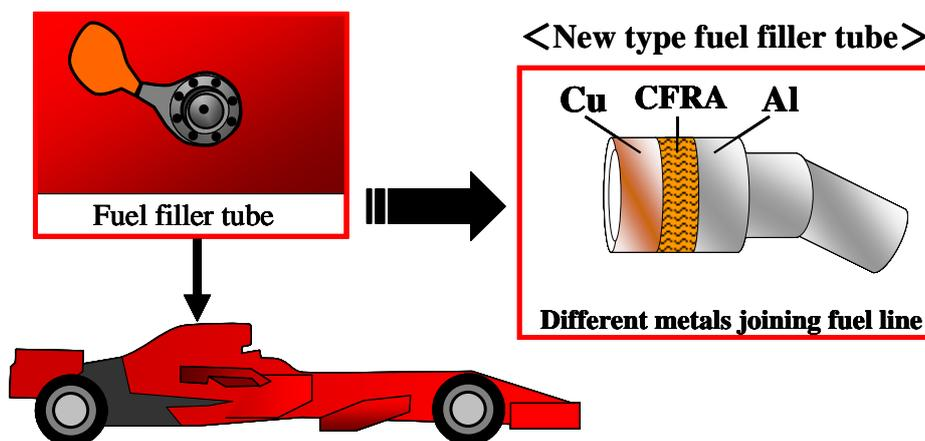
Fig. 1 Schematic diagram of Al/Cu joint new type engines parts.
