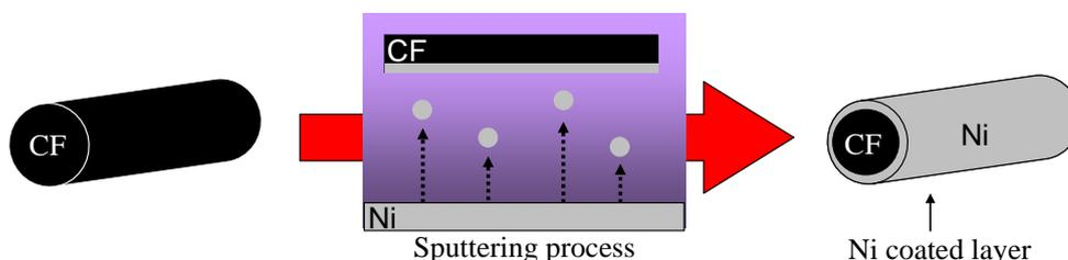
Fig. 2 Schematic drawing of Ni-coating on carbon fiber with DC-magnetron sputtering apparatus.
