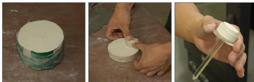
Fig. 2 Sampling process: (a) cutting (b) sampling (c) ready for CT scanning
