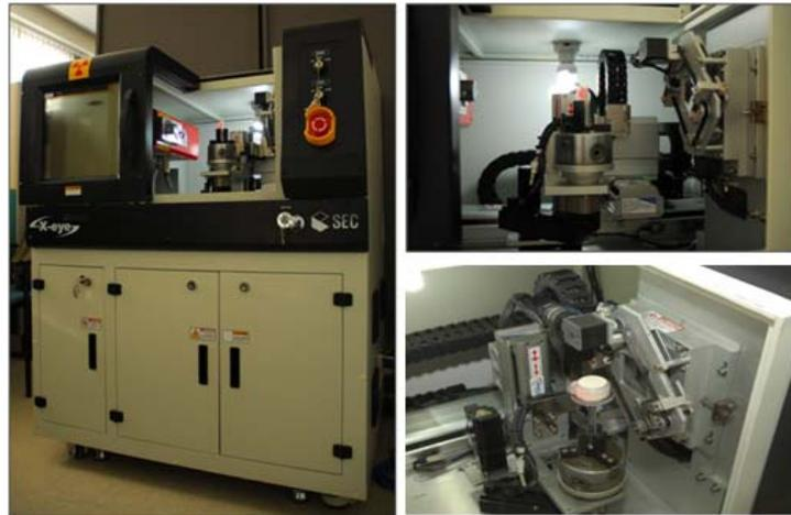
Fig. 1 Micro X-ray CT equipment of KICT (a) view of micro CT scanner (left), (b) arrangement of three major parts (source, manipulator and detector from right hand side, respectively in upper right figure), (c) zoomed manipulator & detector (lower right)
