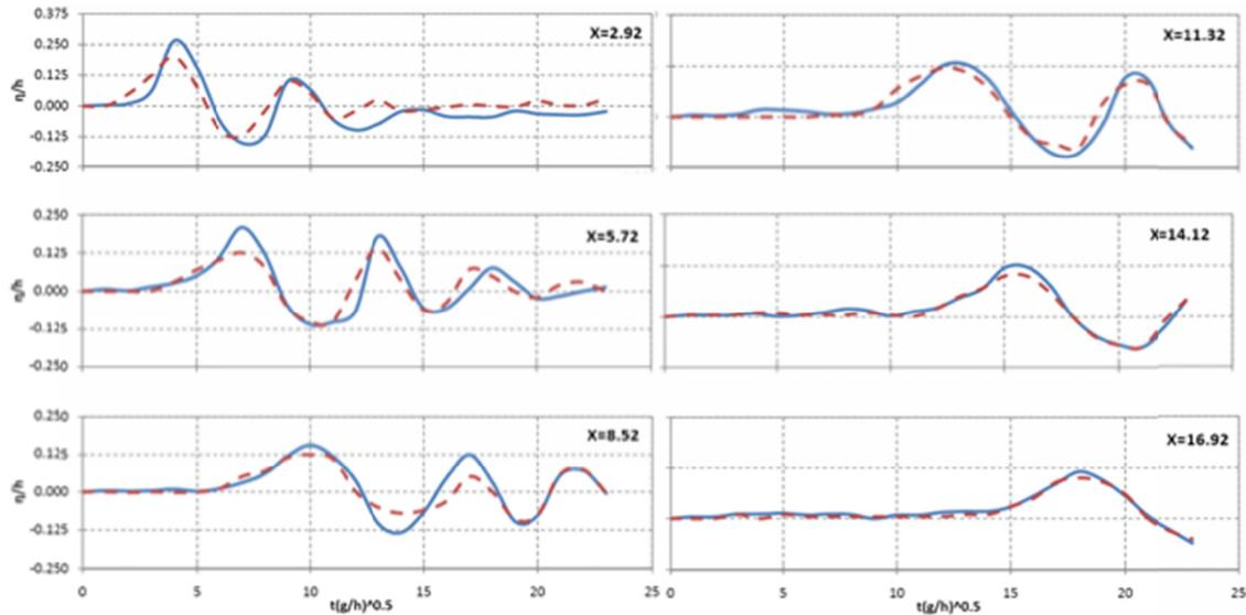
Fig. 4. Wave profile (water surface displacement/depth) comparison between MPS simulation and experimental data
