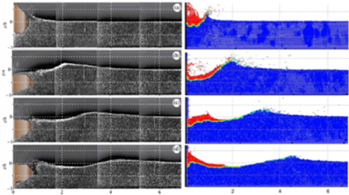
Fig. 3. Snapshot of the particle configuration simulated by MPS model compared with the experimental snapshot for  $Tr=(a)$  0.93, (b) 2.18, (c) 3.42, and (d) 4.67 after slide impact and for the same sequences.
