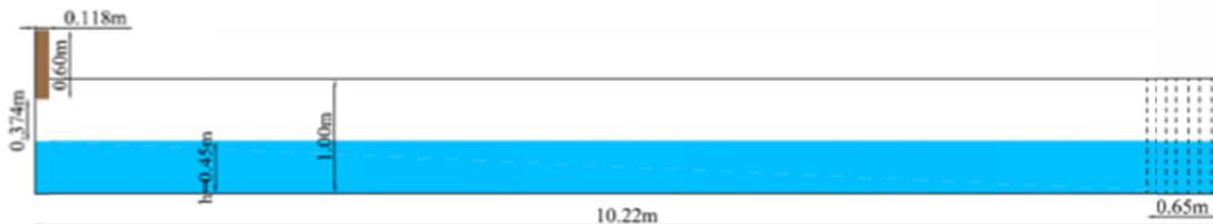
Fig. 2. Sketch of the experimental configuration of sliding box into the water
