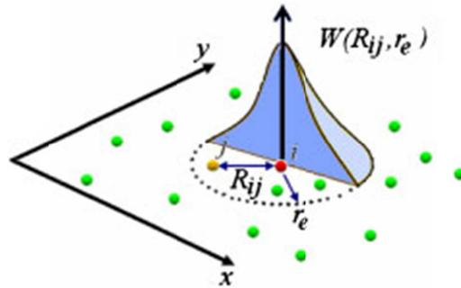
Fig. 1. Particle interaction conceptual model. (Shakibaeinia and Jin 2010)
