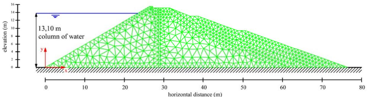
Fig. 5. Finite elements mesh used to discretize the domain of the type cross section in the Gasset dam.
