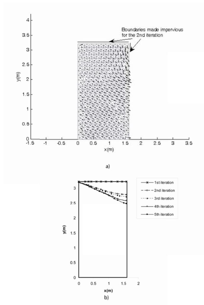
Fig. 1. Iterative procedure employed for computing the free surface in the Muskat problem, changing the impermeability boundary conditions. a) Water velocity vectors after the first iteration, and impermeability boundary conditions for the second iteration. b) Computed free surface after every iteration.
