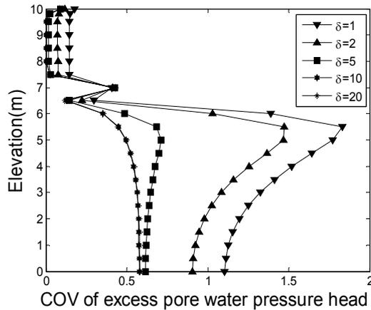
Fig. 9 Effect of correlation length on the COV of excess pore water pressure head ( $t = 1$  s).
