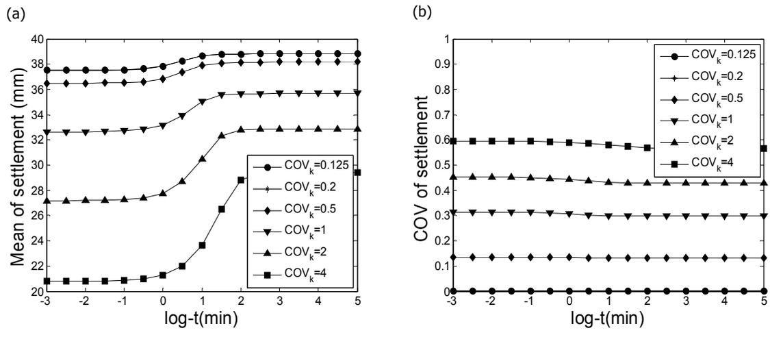
Fig. 4 Effect of  $COV_k$  on the ground settlement
