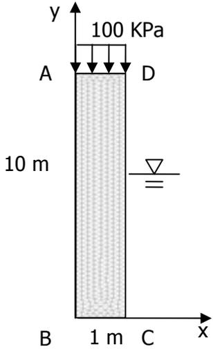
Fig. 1 An illustrative example of unsaturated soil consolidation
