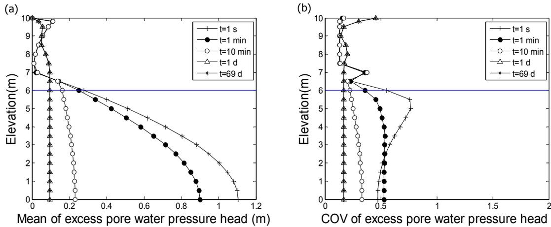
Fig. 2 Variation of excess pore-water pressure head with time ( $COV_k = 0.5$  and  $\delta = 0.1$ )
