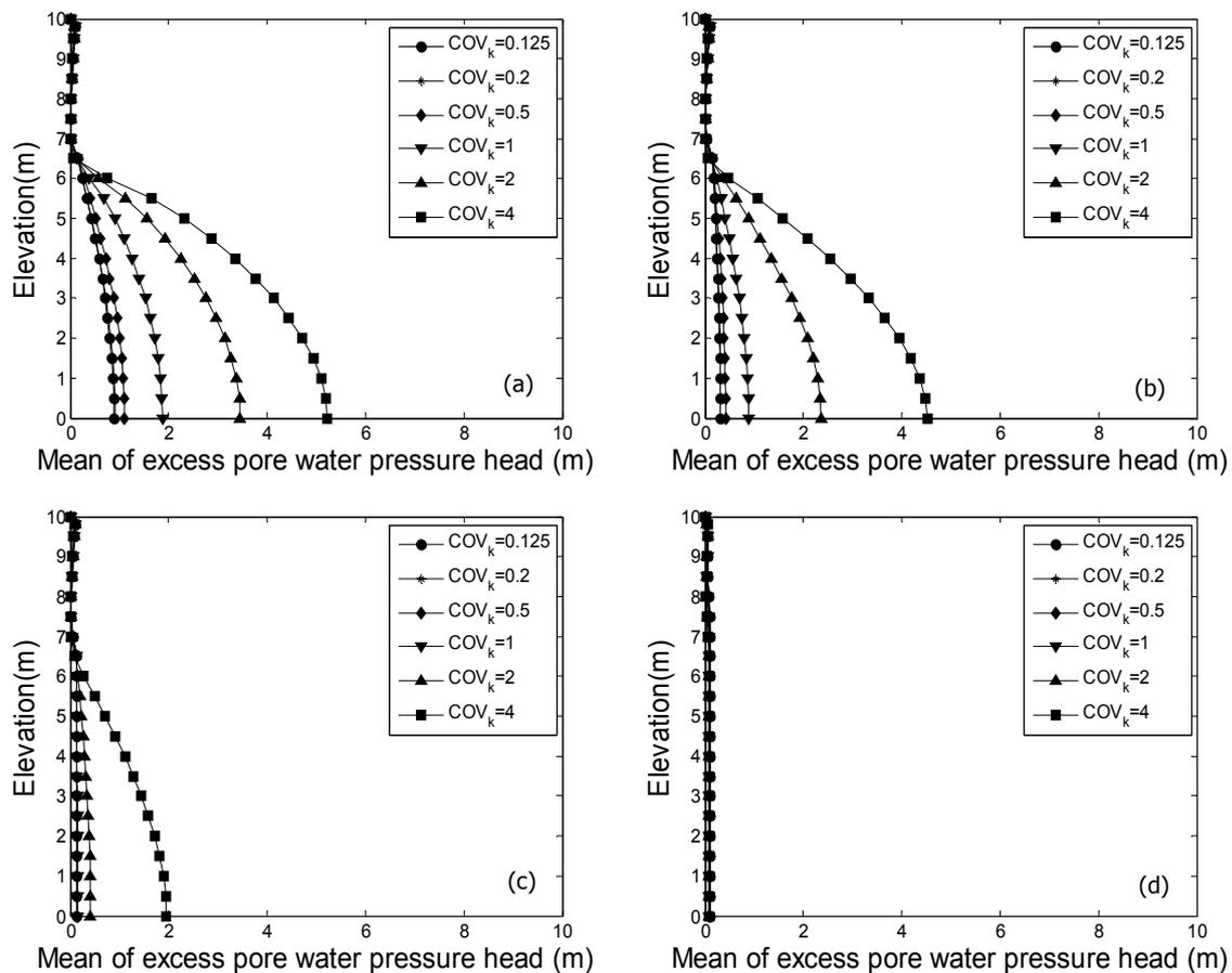
Fig. 5 Effect of  $COV_k$  on mean pore water pressure head profiles:
