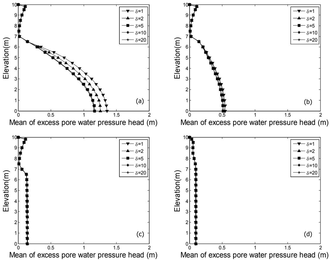
Fig. 8 Influence of correlation length on dissipation of excess pore water pressure head:
