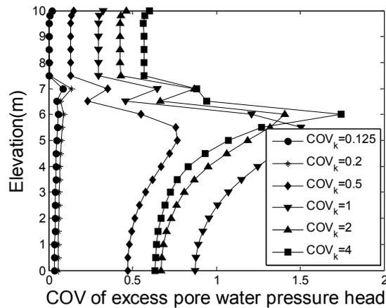
Fig. 6 Effect of  $COV_k$  on the COV of excess pore water pressure head ( $t = 1$  s).
