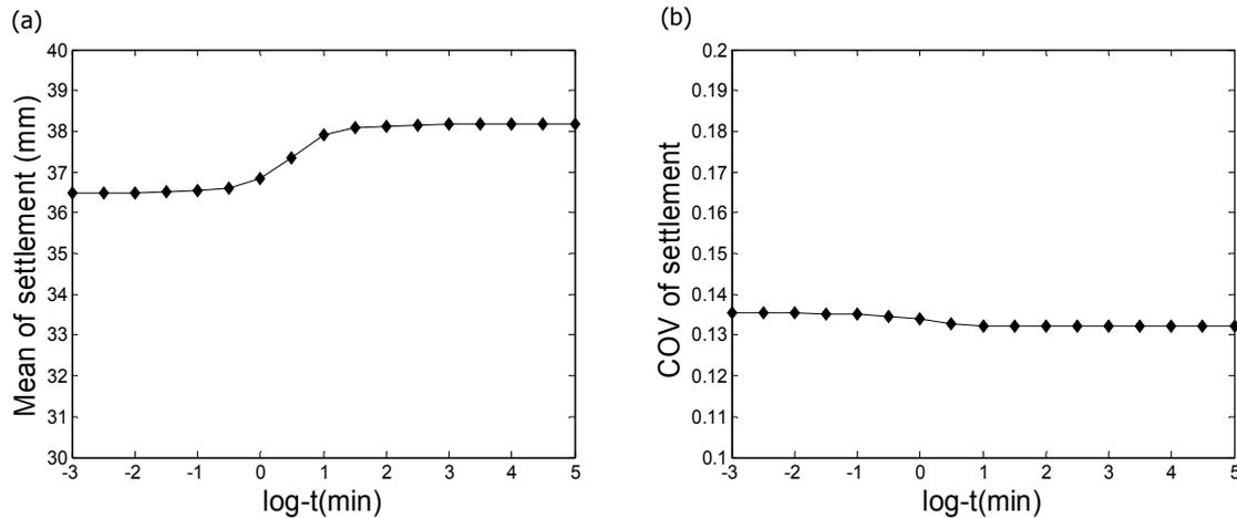
Fig. 3 Variation of ground surface settlement with time ( $COV_k = 0.5$  and  $\delta = 0.1$ ):
