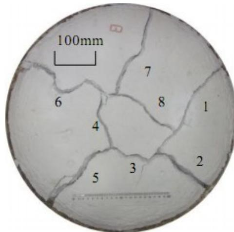
Fig. 2 Stable conditions of the crack and the number of cracks
