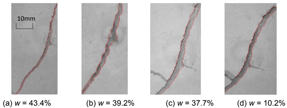
Fig. 3 Development of the first crack at different water contents
