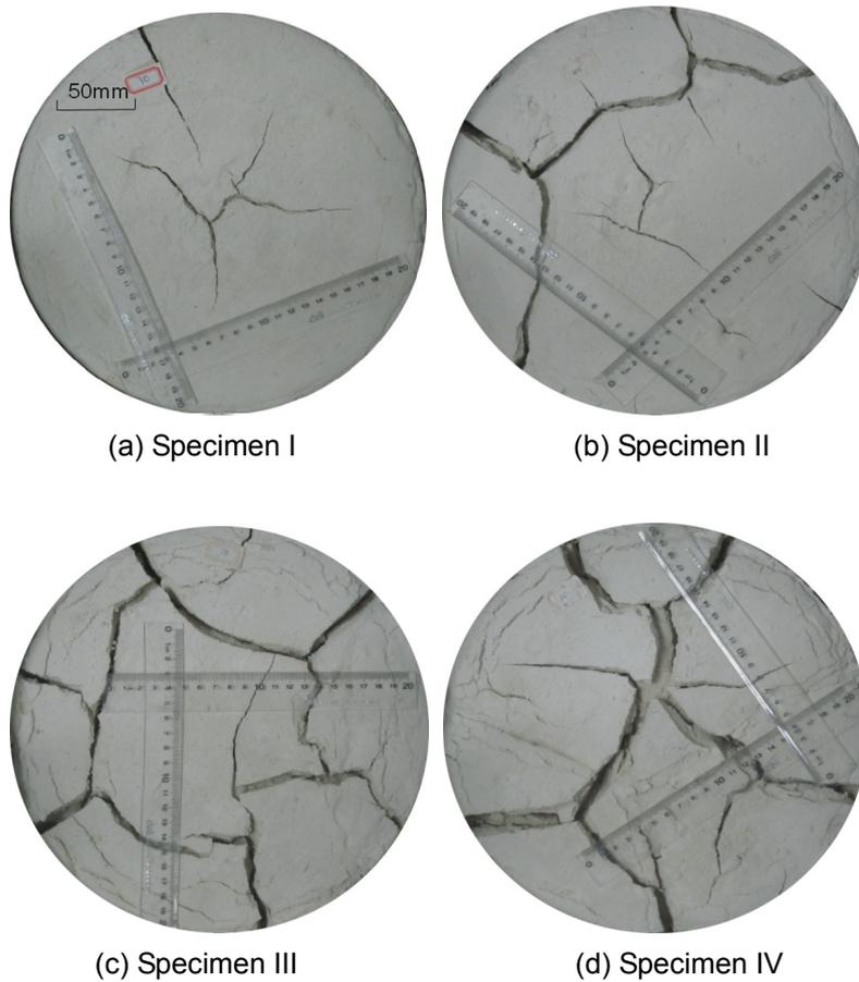
Fig. 7 Four cracked soils with different proportion of montmorillonite at steady state stage
