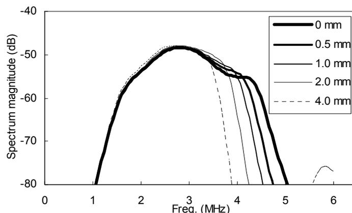
Fig. 4 Performance decrease according to the thickness of the epoxy adhesive layer
