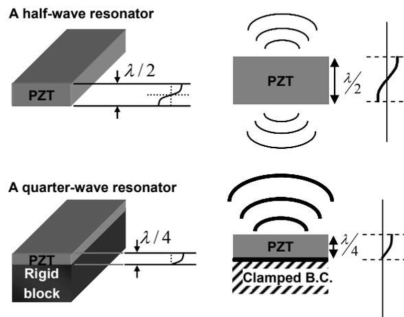
Fig. 1 Normal modes of resonators according to boundary conditions
