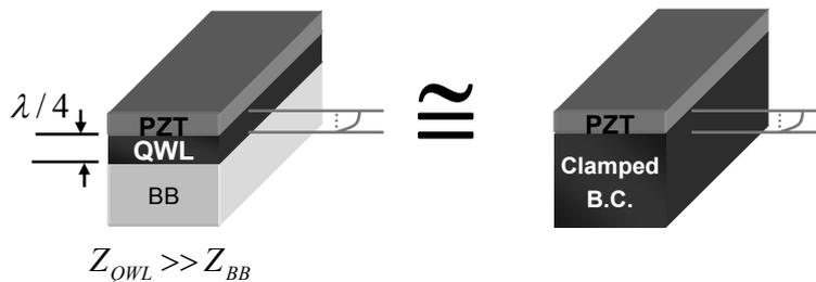
Fig. 2 Principle of a quarter-wave clamped boundary condition
