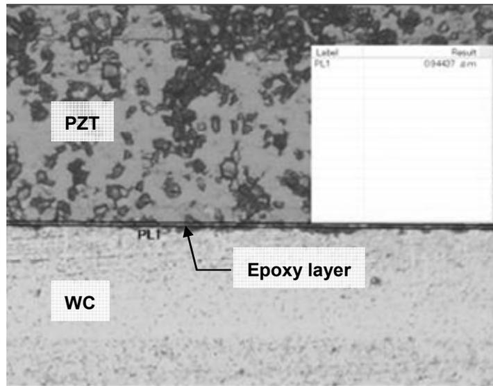
Fig. 6 Section image of epoxy bonding layer between the PZT and the tungsten carbide
