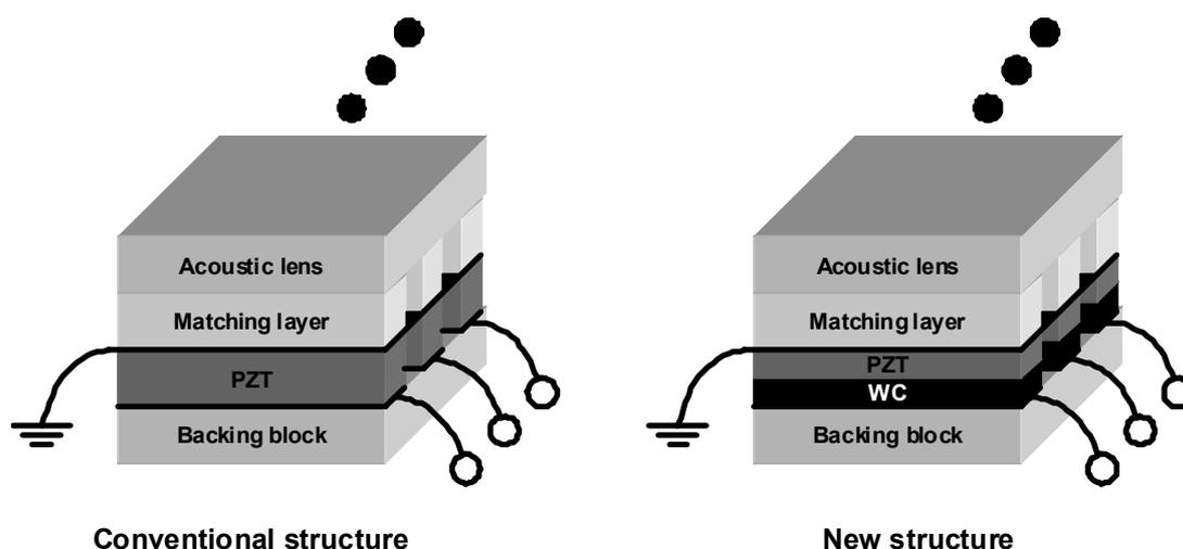
Fig. 5 Array structure of the conventional and new designs
