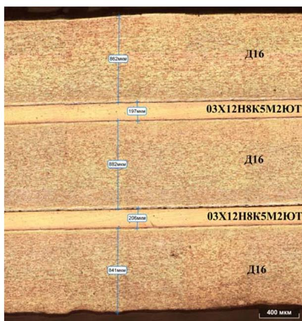
Fig. 3 Microstructure of of the Composite-II
