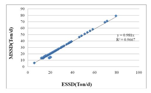
Figure3. Performance of neural network (MLP) in estimation the suspended sediment
