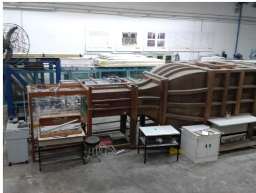
Fig.1. Open-looped wind tunnel at The University of Hong Kong
