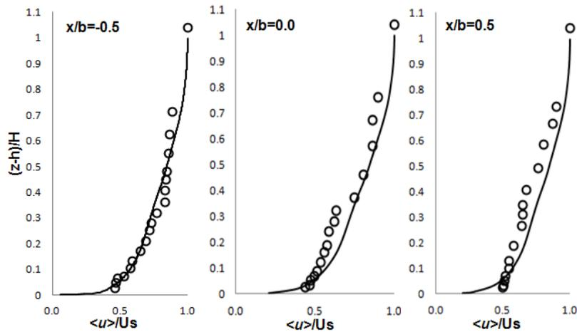
Fig.6. Vertical profiles of the ensemble average streamwise velocity  $\langle u \rangle / U_s$ .
