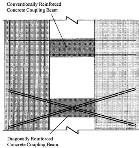
Fig. 1. Rebar pattern for conventional and diagonal reinforcement coupling beams.
