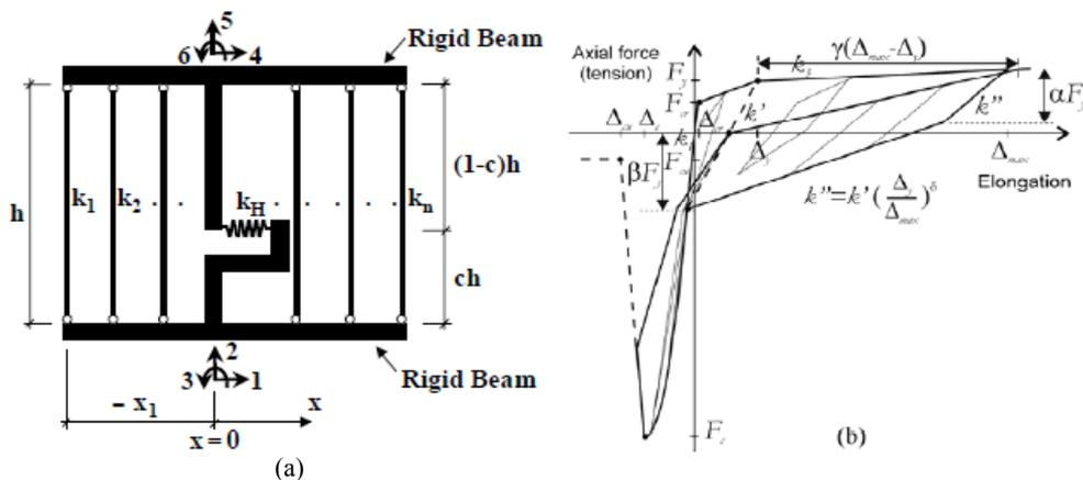
Fig. 4. Multiple Vertical Line Element Model (MVLEM) (Orakcal et al., 2006)
