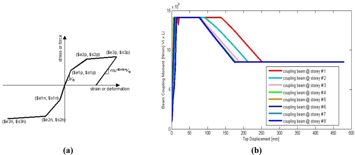
Fig. 7. The Hysteretic Model in OpenSees (left) and the beam moment distribution (right)
