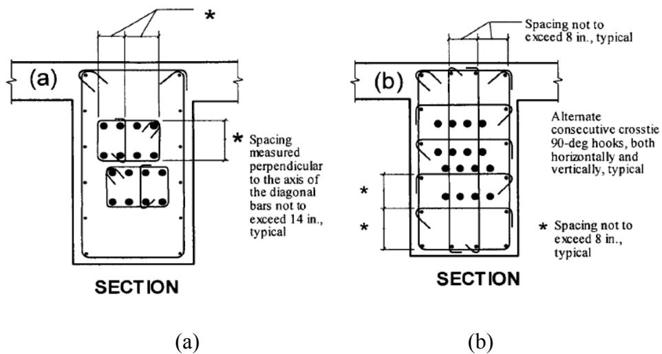
Fig. 2. Confinement alternatives provided in ACI 318-05 and ACI 318-08.
