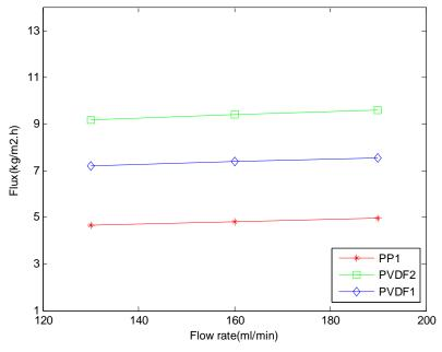
Figure 1. Effect of feed flow rates on flux
