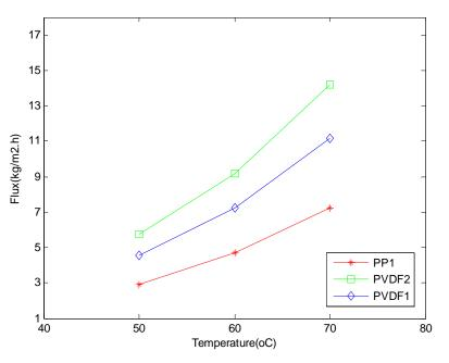
Figure 2. Effect of feed temperature on flux for different membranes
