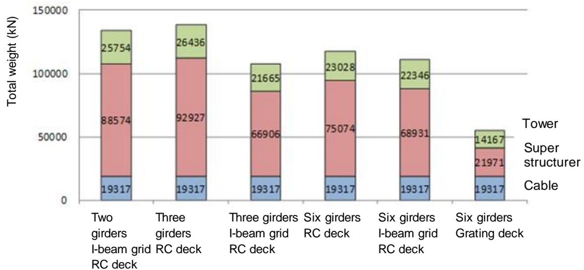
Fig. 3 Comparison of total weight (Hanger interval of 15m)
