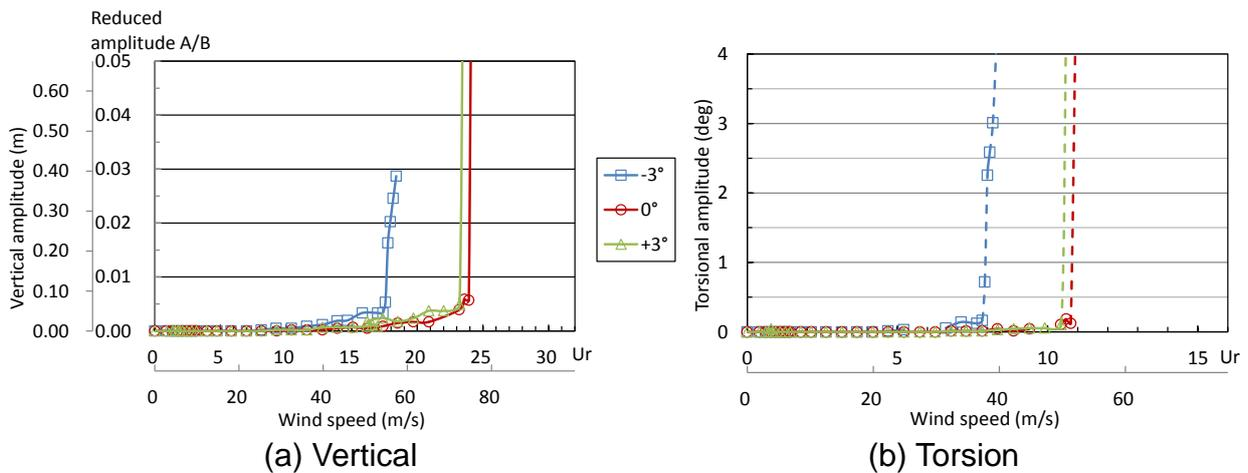
Fig. 11 Vibration amplitude vs. wind speed (Case 14)
