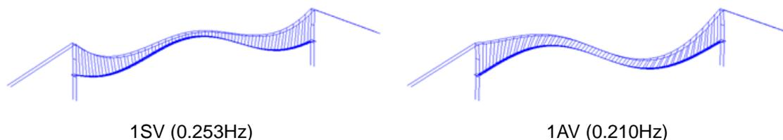
Fig. 4 Vibration mode shapes (No.11: 15-6-I)
