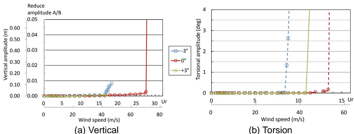
Fig. 12 Vibration amplitude vs. wind speed (Case 20)
