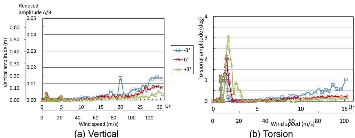
Fig. 7 Vibration amplitude vs. wind speed (Case 1)
