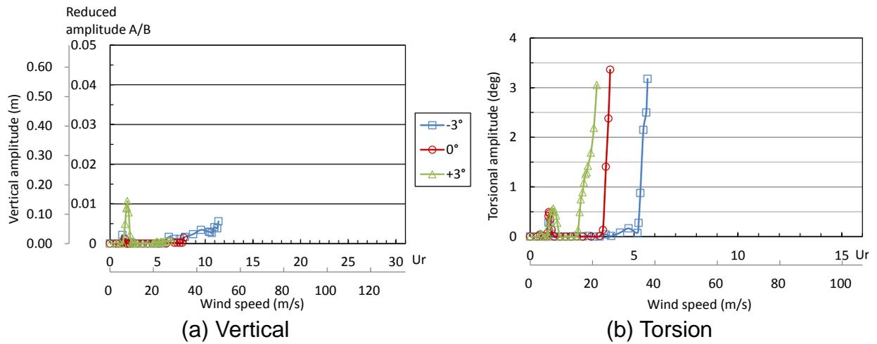
Fig. 9 Vibration amplitude vs. wind speed (Case 4)
