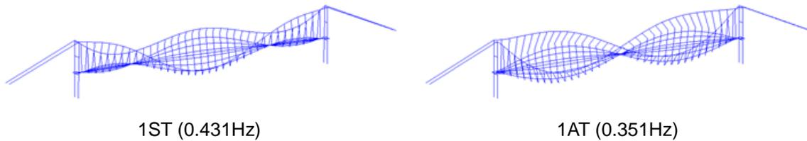
Fig. 4 (cont.) Vibration mode shapes (No.11: 15-6-I)
