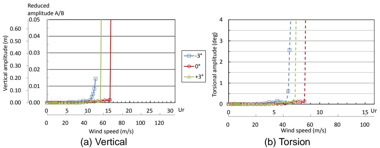
Fig. 10 Vibration amplitude vs. wind speed (Case 7)
