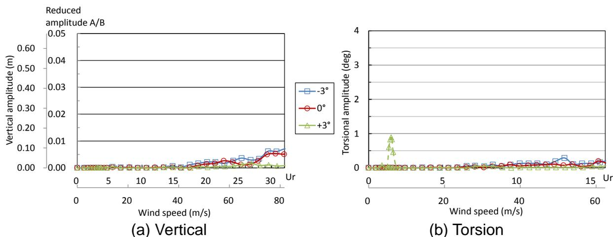
Fig. 8 Vibration amplitude vs. wind speed (Case 15)
