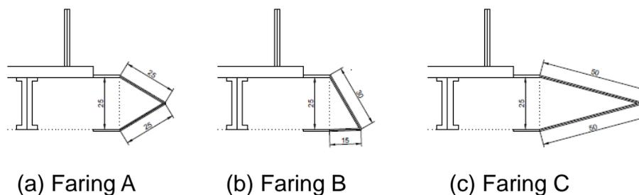
Fig. 6 Types of aerodynamic countermeasure
