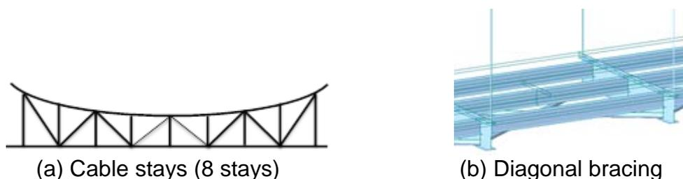
Fig. 13 Structural countermeasures
