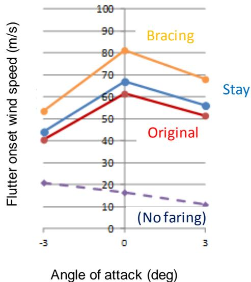
Fig. 14 Flutter onset wind speed for structural countermeasures
