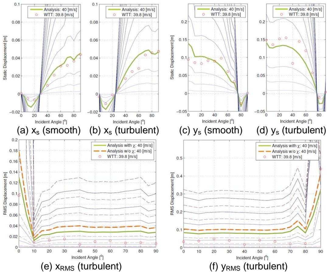
Fig. 6 Static and RMS response of the tower in erection stage (2D model)
