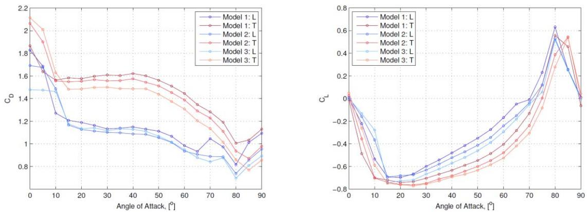
Fig. 3 Steady state wind load coefficients
