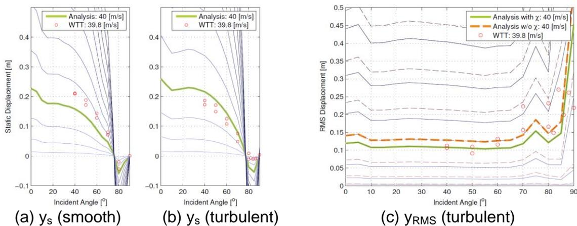
Fig. 8 Static and RMS response of the tower in service stage (3D model)
