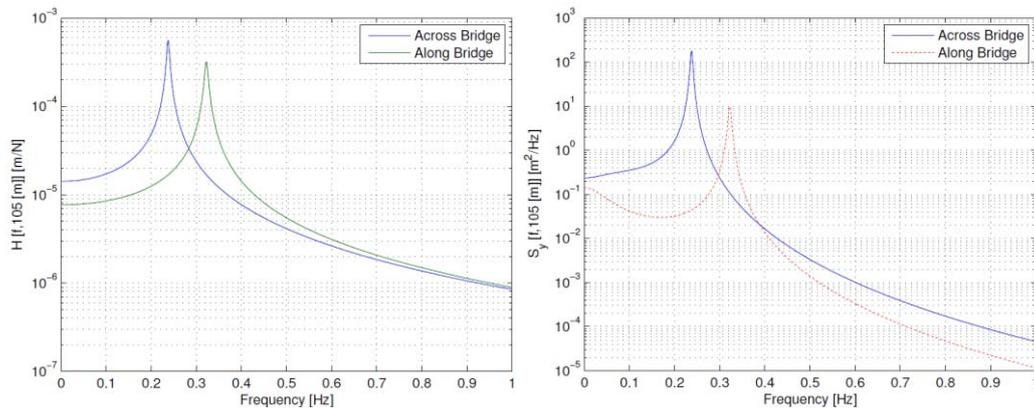
Fig. 5 Frequency response function and power spectrum of response
