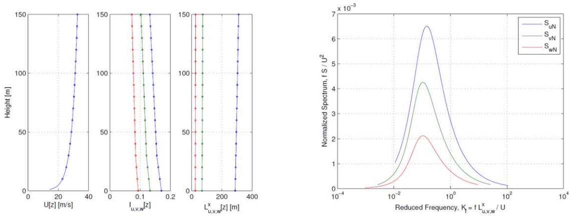
Fig. 1 Wind velocity, turbulence intensity, length scale and PSD of wind speed
