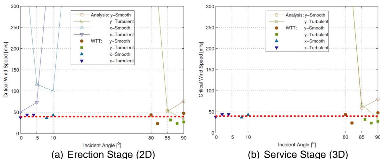
Fig. 4 Flutter stability analysis of the tower
