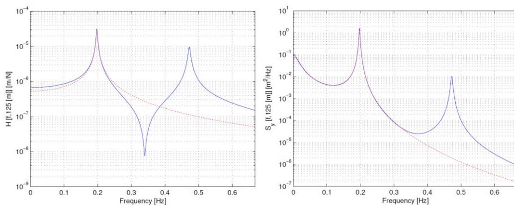
Fig. 7 Frequency response function and PSD of the response of the tower
