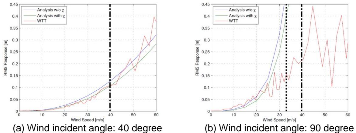
Fig. 9 RMS response of the tower in service stage as a function of wind speed
