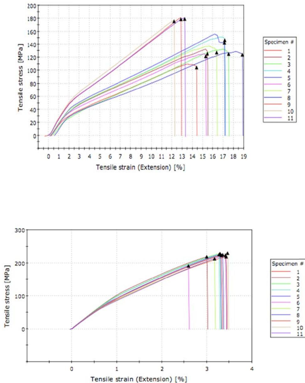
Fig. 1 Stress-strain curves of E-glass/epoxy (top) and PEEK CF40 tensile specimens (bottom)
