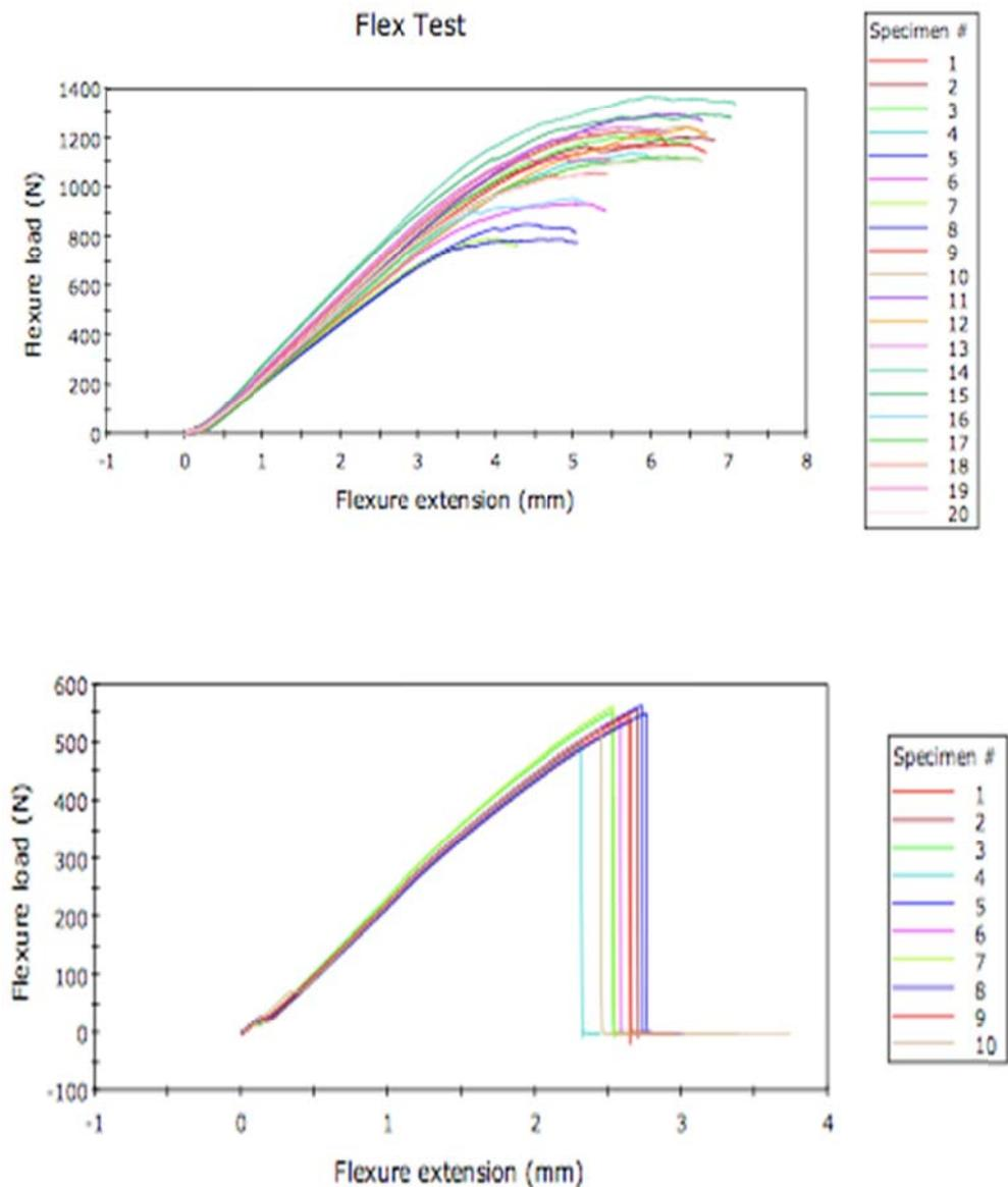
Fig. 2 Load-displacement curves of E-glass/epoxy (top) and PEEK CF40 flexural specimens (bottom)
