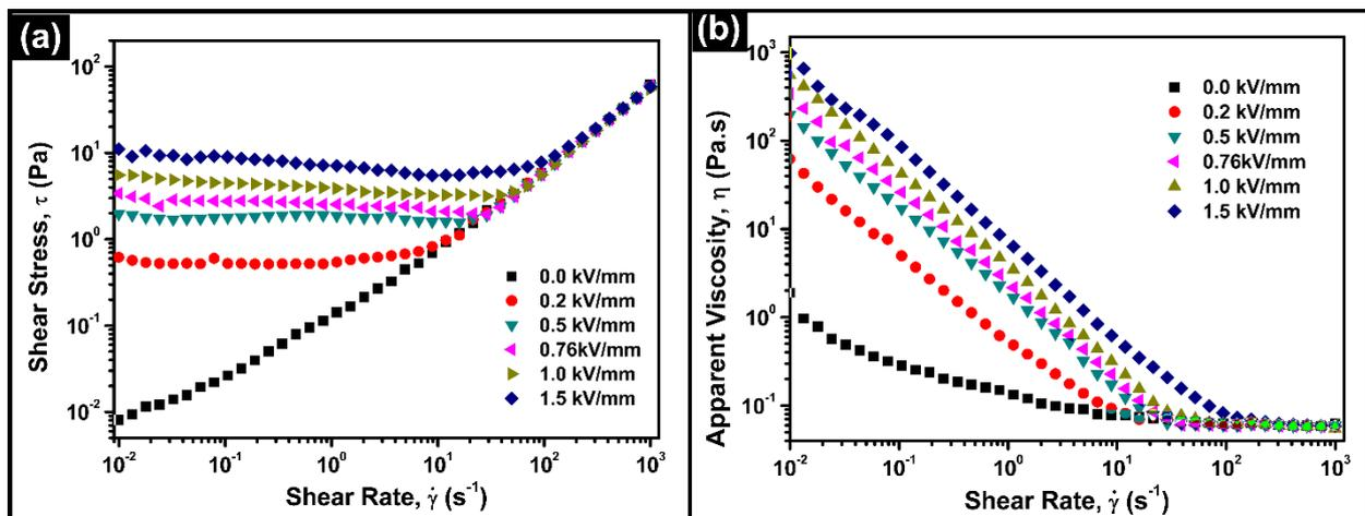
Fig. 2 The flow curves for the ER suspension with PAV-R as dispersed phase.
