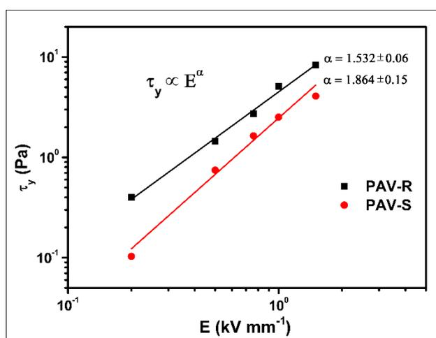
**Fig. 3** Yield stress as a function of the applied electric field strengths.
