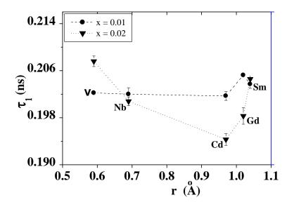
Fig. 7. Variation of lifetime  $\tau_1$  with the ionic radii for x = 1 % and 2 %
