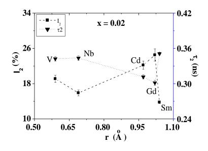
Fig. 1 The variation of relative intensity  $I_2$  and the lifetime  $\tau_2$  with the ionic radii of the ions substituted Li-ferrite.
