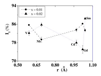
Fig. 6. Dependence of the relative intensity  $I_1$  with the ionic radii for x = 1 % and 2 %
