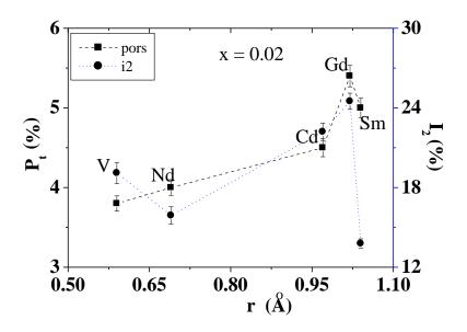
Fig.2. Variation of the total porosity and  $I_2$  % as a function of the ionic radii of the substituted ion.
