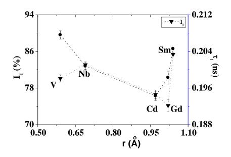
Fig.3. Dependence of the relative intensity  $I_1$  and lifetime  $\tau_1$  with the ionic radii of the substituted ions.
