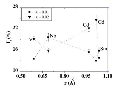
Fig. 8. Variation of the relative intensity  $I_2$  with the ionic radii for x = 1 % and 2%
