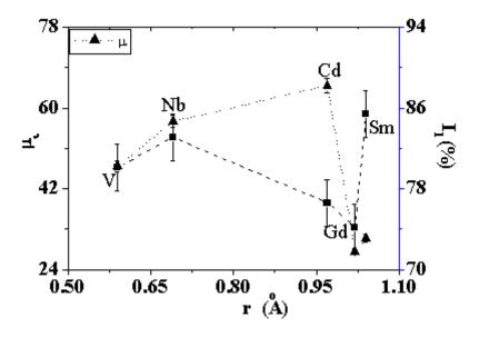
Fig. 5 The dependence of the initial permeability  $\mu_i$  and  $I_1$  on the ionic radii of the ions substituted Li-ferrite
