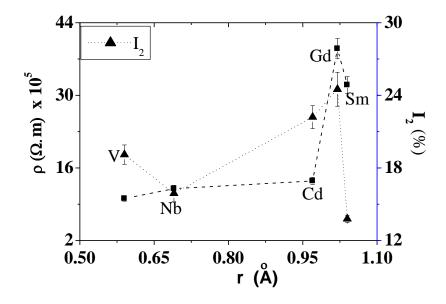
Fig. 4 Variation of the electrical resistivity  $\rho$  and  $I_2$  % against the ionic radii of the substitute ions for Li-ferrite.
