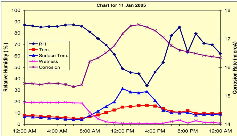
Figure 6. Atmospheric data for Sabia on 10 & 11 January 2005, showing two days hourly profiles of RH, Temperature, Surface Temp, wetness, and corrosion rate
