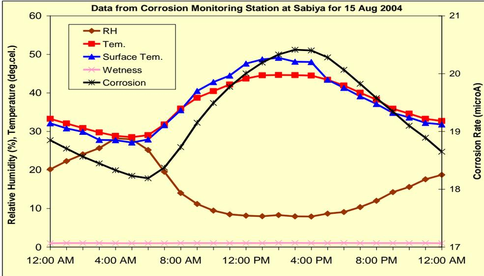
Figure 5. Atmospheric data for Sabia on 15 August showing one day profile of RH, Temperature, Surface Temp, wetness, and corrosion rate
