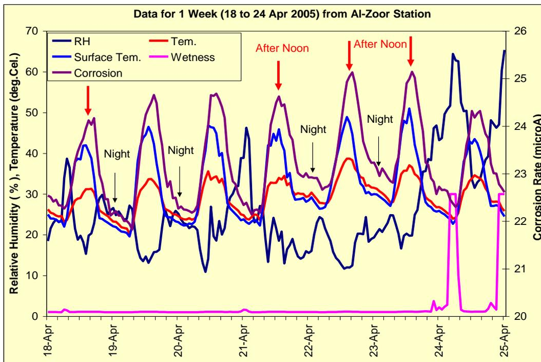
Fig. 7. Atmospheric data for Al Zoor area on 25 February & 18 to 24 April 2005, showing (a) one days and (b) two weeks hourly profiles of RH, Temperature, Surface Temp, wetness, and corrosion rates
