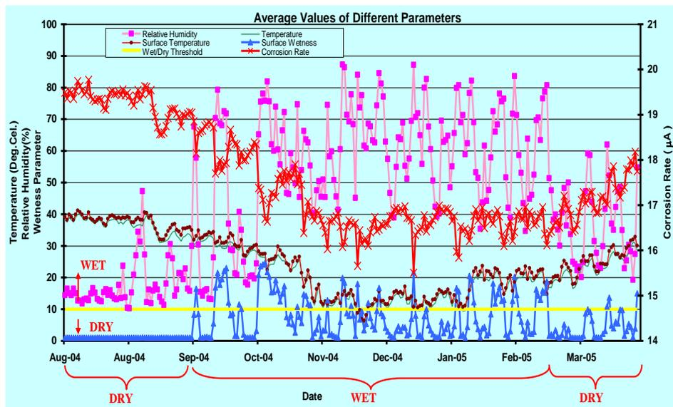
Figure 3. Atmospheric Corrossivity data for Sabia Station North of Kuwait, showing, bimetallic corrosion, TOW, R.H, surface temperature and air temperature
