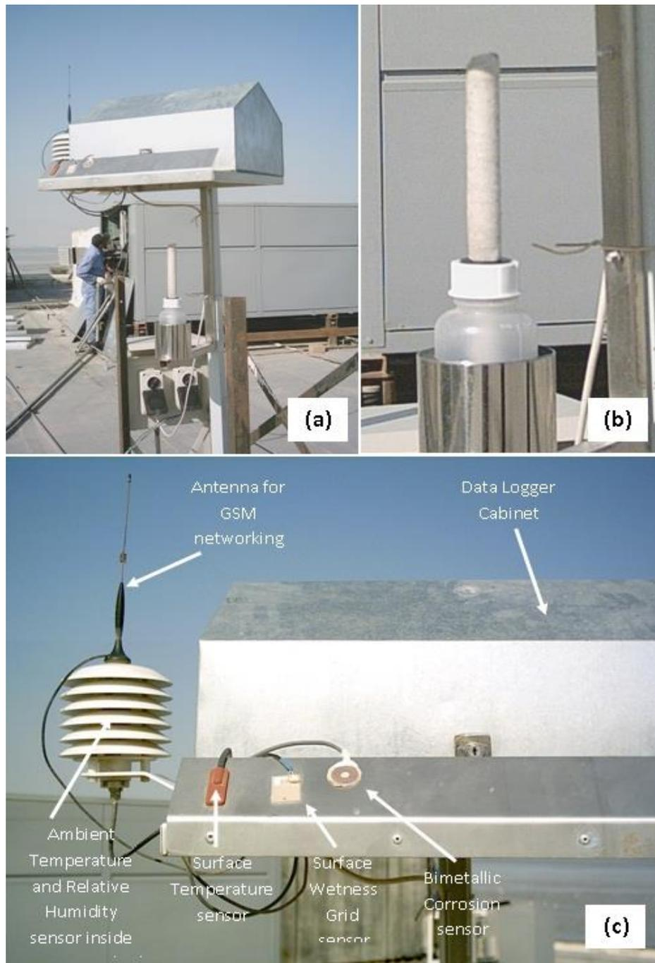
Figure1 Atmospheric Corrosivity Monitoring Station in Kuwait. (a) Overall view on site. (b) Salt Candle and (c) Close-up to reveal sensors.
