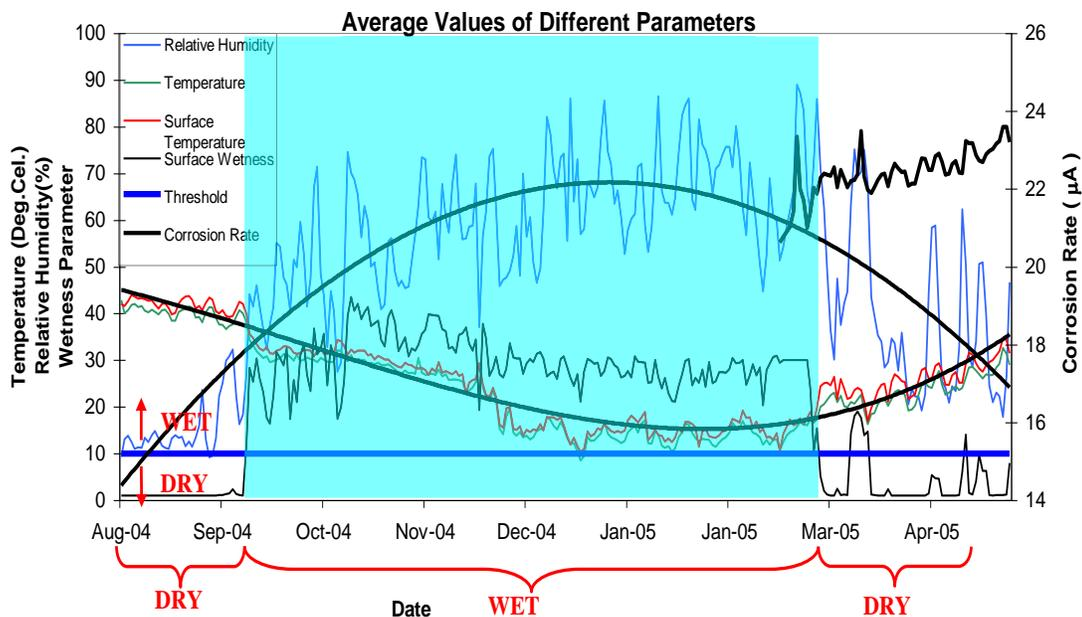
Figure 4. Atmospheric Corrossivity data obtained for Al-Zoor Texaco Station Site South of Kuwait, showing, bimetallic corrosion, TOW, R.H, surface temperature and air temperature.
