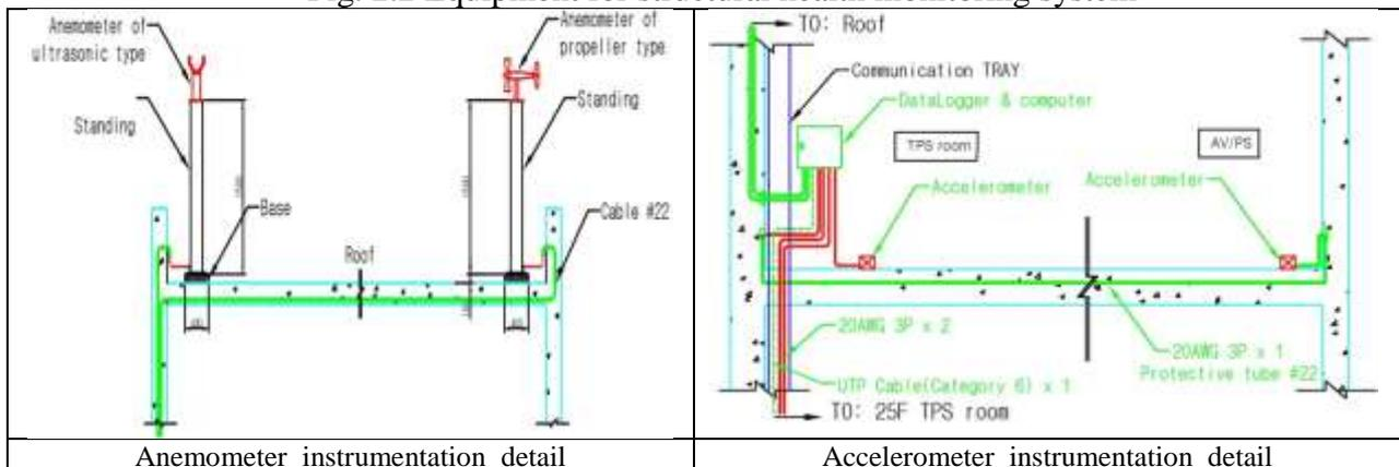
Fig. 2.3 Instrumentation detail installed for Structural health monitoring system
