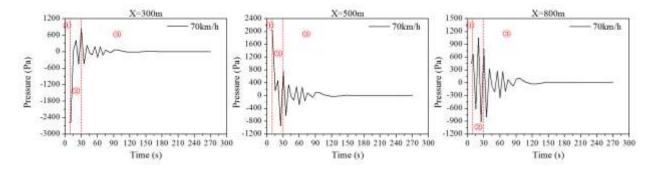
Fig.4 Pressure variation with time of three typical locations
