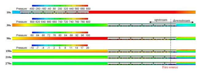
Fig.3 Pressure around train varying with time
