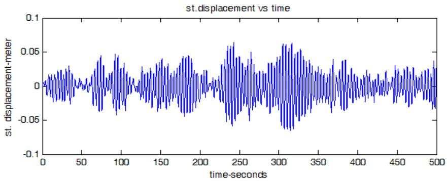
Fig.8 Along-wind responses with ATMD ( $\mu_{AP}=0.3$ , rms=0.0210)
