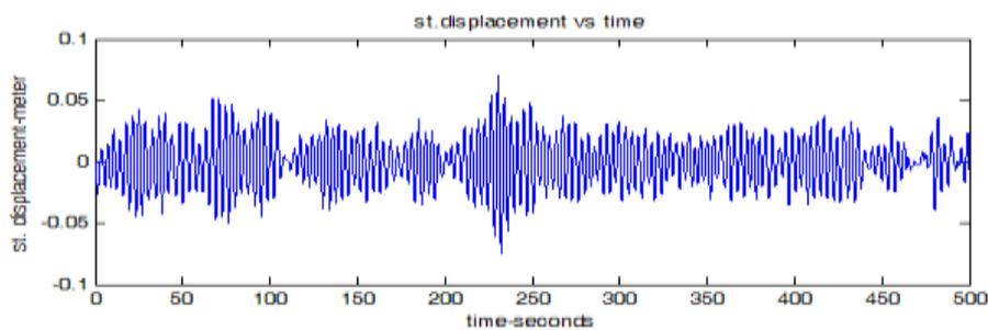
Fig.5 Along-wind responses with ATMD ( $\mu_{AP}=0.03$ , rms=0.0200)
