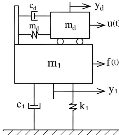
Fig. 1: Building-ATMD system
