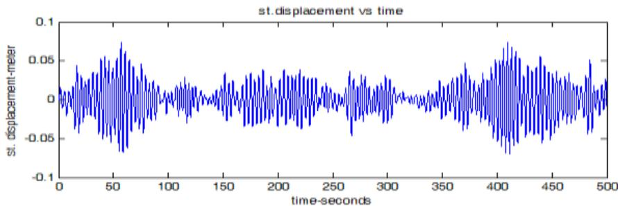
Fig.4 Along-wind responses with ATMD ( $\mu_{AP}=0.01$ , rms=0.0222)
