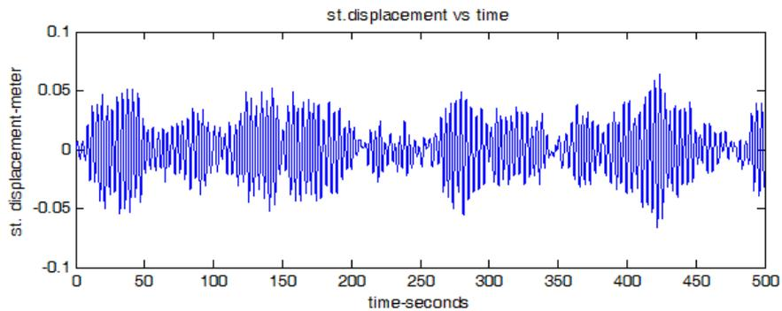
Fig.9 Along-wind responses with ATMD ( $\mu_{AP}=0.5$ , rms=0.0216)
