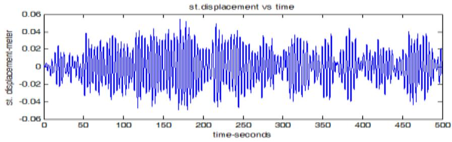
Fig.6 Along-wind responses with ATMD ( $\mu_{AP}=0.05$ , rms=0.0196)
