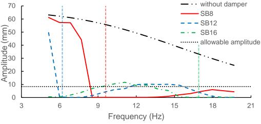
Fig. 1 Amplitude of the hanger vibration
