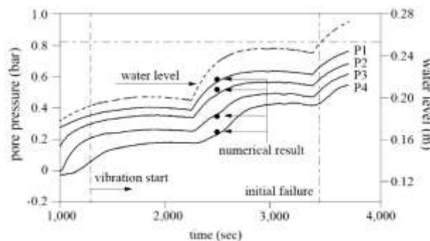
Fig. 7 Numerical results and comparison with centrifuge test
