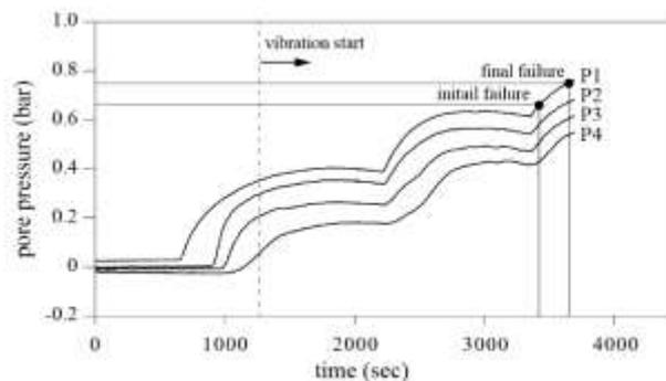
Fig. 4 Results of centrifugal model test (Park 2015)
