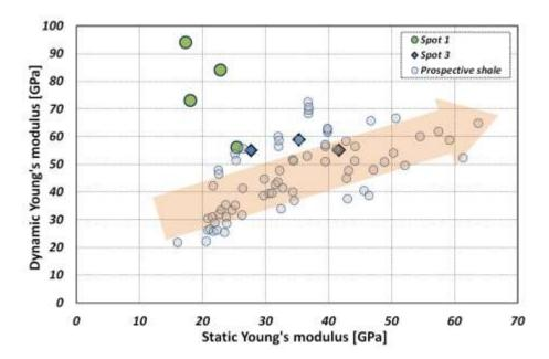
Fig. 4 Correlation between dynamic Young's modulus and static Young's modulus of shale in Gyeongsang Basin and comparison with the shale of Britt and Schoeffler (2009)
