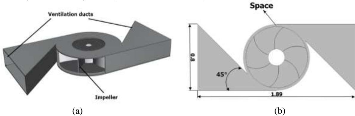
**Fig. 1** Model of the turbine: (a) three-dimensional; (b) sectional, unit: m
