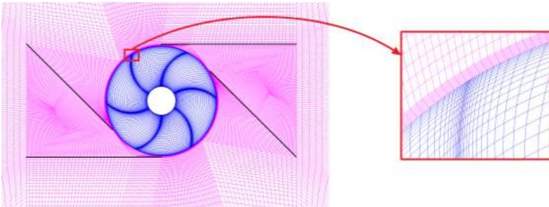
Fig. 3 Mesh of the flow field
