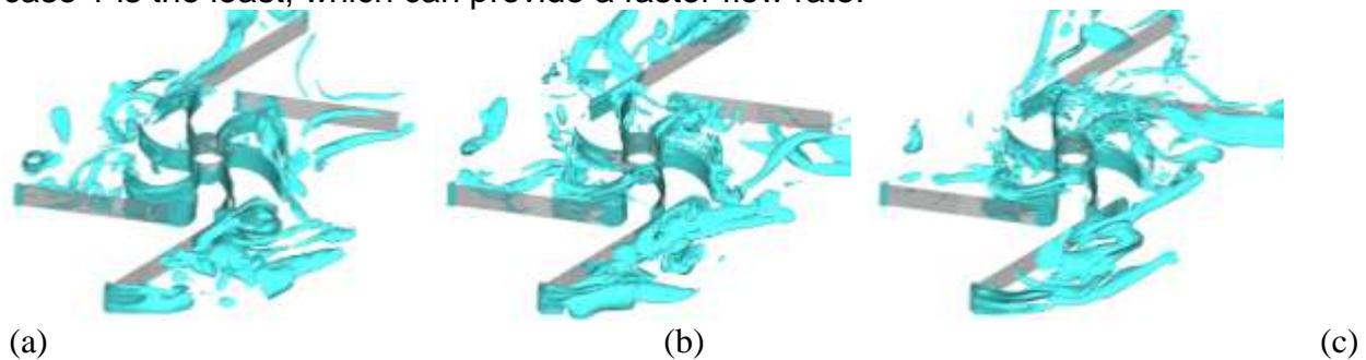
Fig. 9 Vorticity isosurface at  $Q=500$  of: (a) Case 1; (b) Case 2; (c) Case 3
