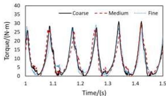
**Fig. 5** Comparison of meshes
