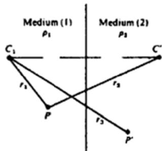
Fig. 1 Image electrode near the boundary (Telford et al., 1990)
