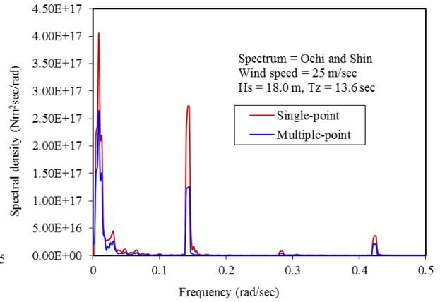
Fig. 7 PSD of bending moment response under high sea state
