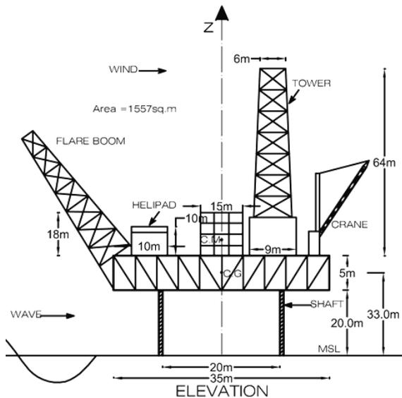
Fig. 4 Full scale dimensions of tower superstructure
