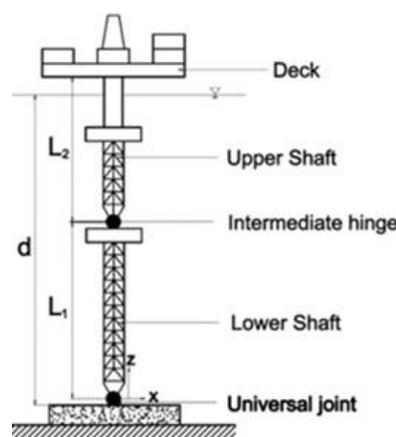
Fig. 1 Schematic of double hinged articulated tower
