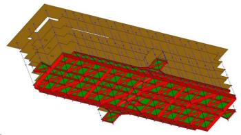
Figure 1. 3D view of building showing the upper structure and supported SNSF foundation system.
