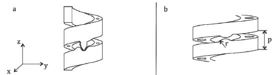
Fig. 2 schematic view of contours for the helix. Involute (a) and unrolling circles (b)
