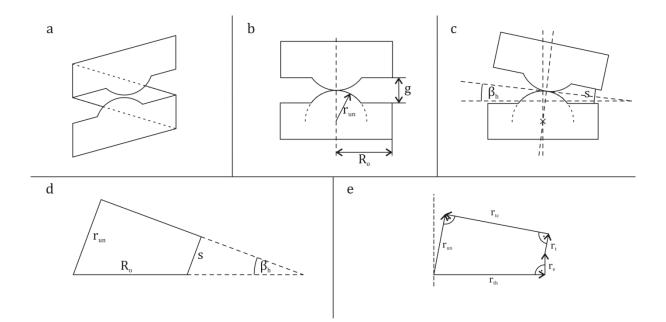
Fig. 5 Schematic view of helical joint (a), simplified model (b), half bending angle β<sub>h</sub> and tendon lengths (c), approximation (d) and closed vector chain (e)
