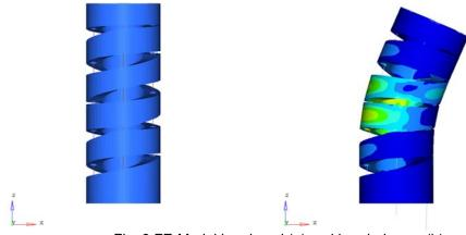
Fig. 3 FE-Model in relaxed (a) and bended pose (b)
