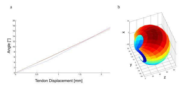
Fig. 6 comparison of bending angle with different approaches. FEM (blue), exact analytical approach (red) and linearized approximation (green) (a). Working space for the proposed design (b)
