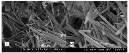
Fig. 3 SEM images of (a,b) untreated and (c,d) plasma treated clinoptilolite.
