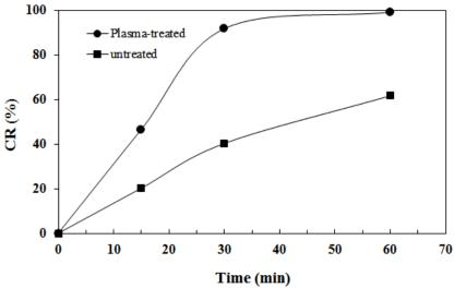
Fig. 4 The potential of untreated and plasma untreated catalysts on decolorization process (pH=5, 3 mmol/L  $H_2O_2$ , 20 mg/L dye concentration and 2 g/L catalyst).
