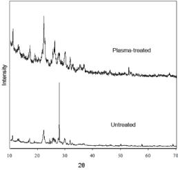
Fig. 2 The XRD patterns of untreated and plasma treated clinoptilolite
