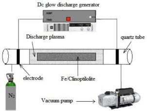
Fig.1 Schematic diagram of the plasma catalyst treatment using glow discharge
