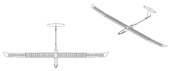
Fig. 1 Simplified configuration of EAV-2
