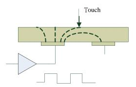
Fig. 1 Projected capacitive touch technology to capture from the electrode.
