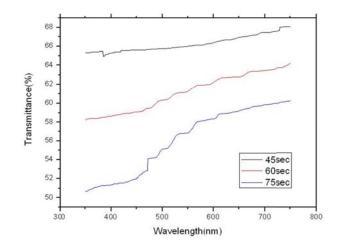
Fig. 5 Transmittance of samples for different deposited time.
