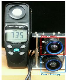
Fig1. Camera configuration for exposure control
