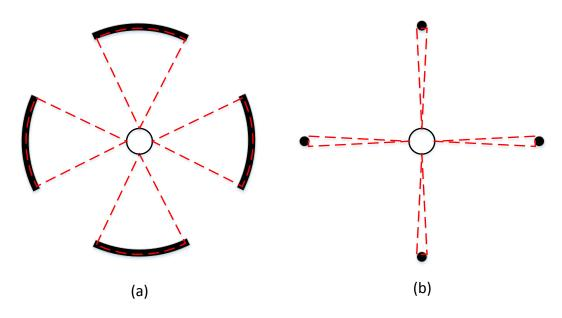
Fig. 1 (a) General ultrasonic sensor model. (b) Special ultrasonic sensor used in this paper.
