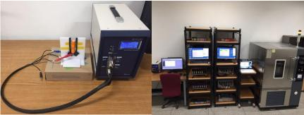
Fig. 2 Elctrochemical and electrical set for test of Li-ion cells
