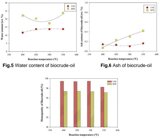
Fig.7 Homogeneity of biocrude-oil
