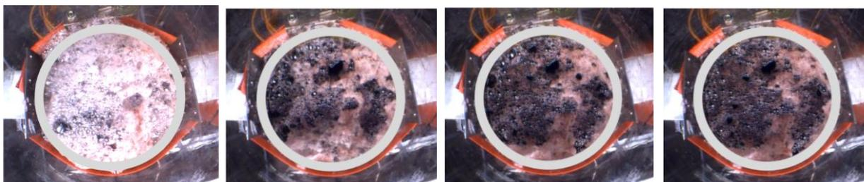
Figure 12: Visual evaluation of the foam decay with frequencies 80, 120 & 250 kHz from test start in 5 second steps (from left to right).
