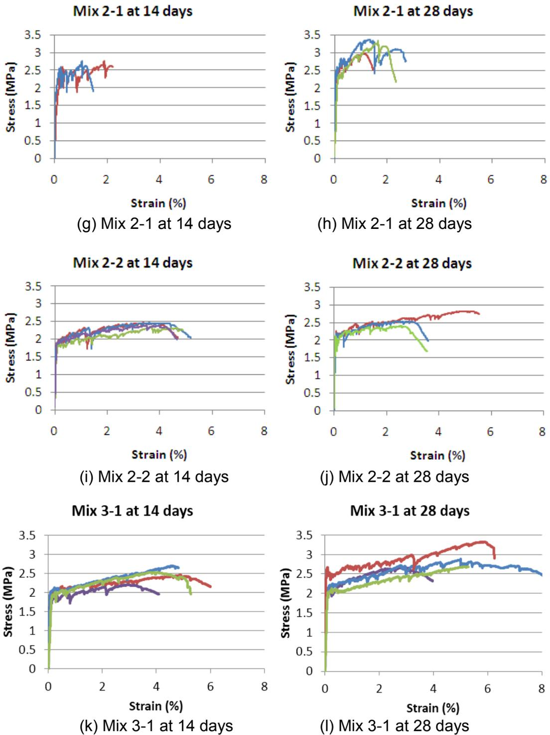
Fig. 5. Tensile stress and strain curves (continued)
