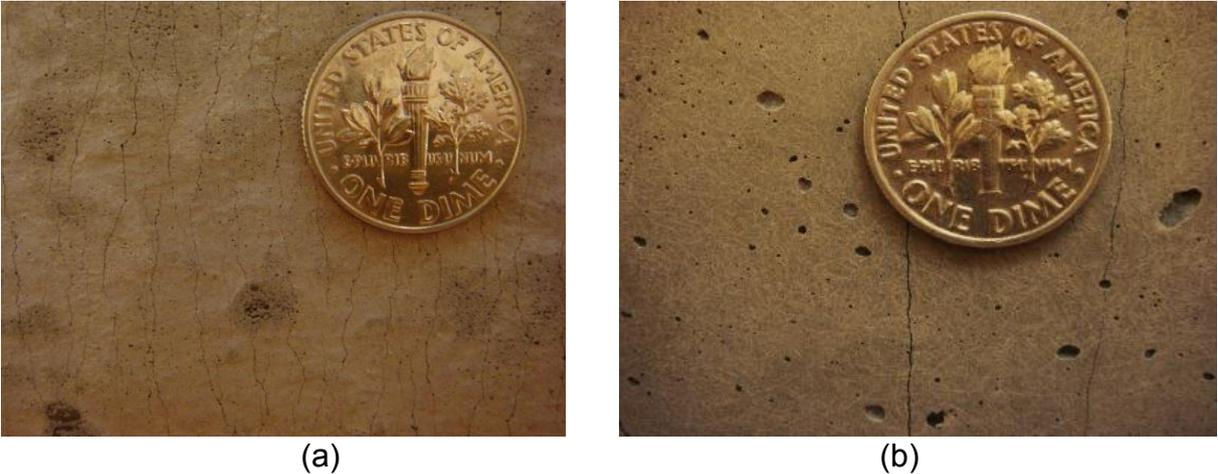
Fig. 4. Specimen surface; (a) Mix 1-1 (homogeneously distributed many tiny air bubbles); (b) Mix 2-1 (normal entrapped air bubbles)
