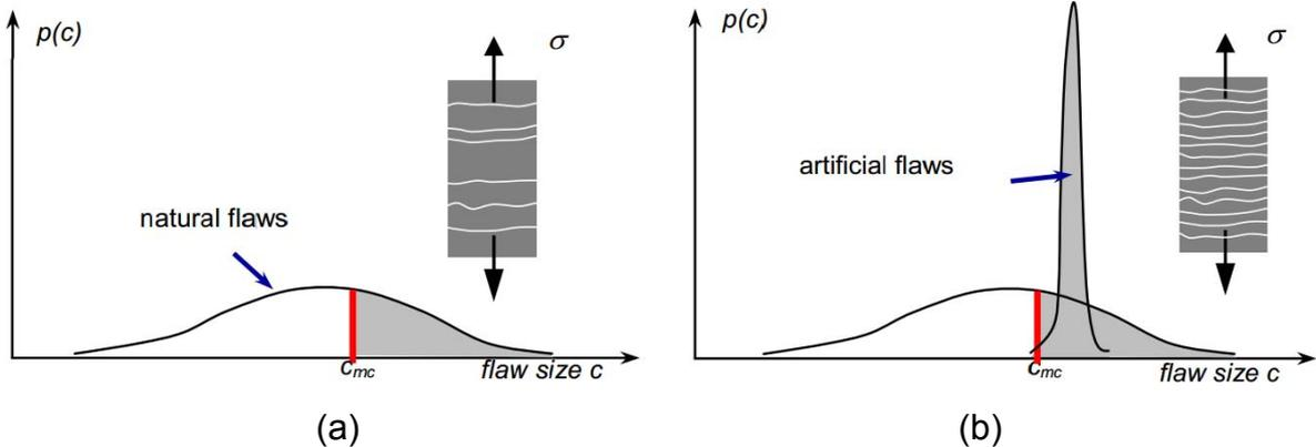
Fig. 1. Scheme of the flaw size tailoring for saturated multiple cracking in fiber reinforced brittle matrix composites: (a) natural flaw size distribution with random nature inherent from processing; (b) artificial flaws larger than critical size  $c_{mc}$  imposed to ensure saturation of multiple-cracking (Wang and Li 2004).
