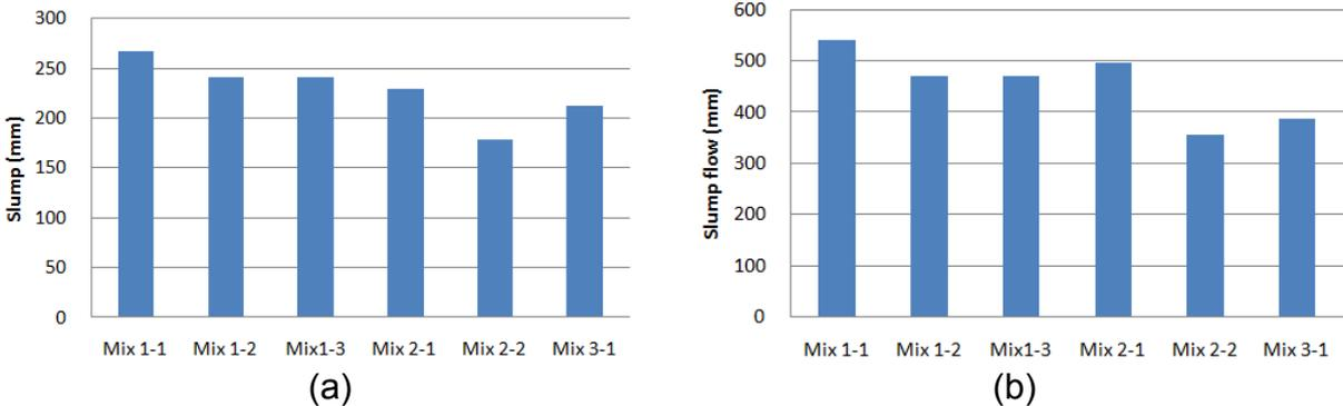
Fig. 2. Flowability: (a) slump and (b) slump flow
