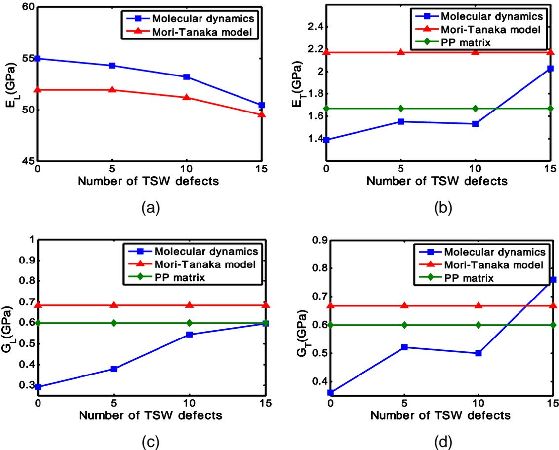
Fig. 2 Transversely isotropic elastic moduli of CNTs reinforced composites (a) longitudinal Young's modulus (b) Transverse Young's modulus (c) Longitudinal shear modulus (d) In-plane shear modulus.
