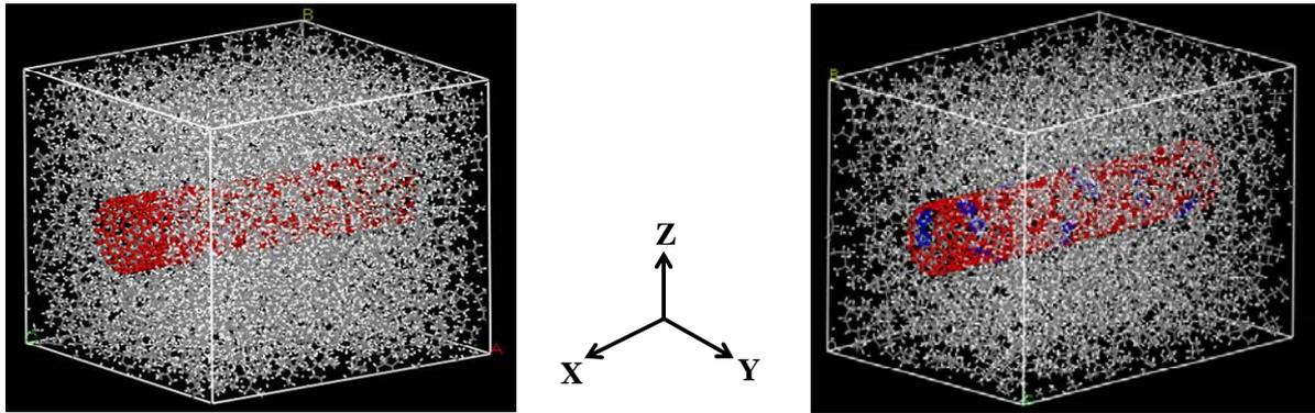
Fig. 1 Transversely isotropic nanocomposites unit cell structure, left: pristine CNT right: 10 TSW defected CNT
