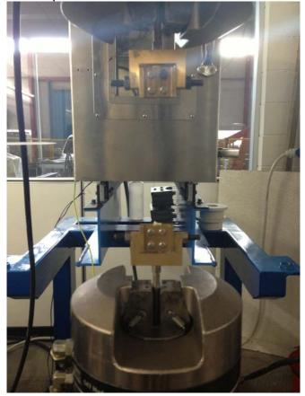
Fig. 1 Universal testing machine: detail of the additional devices used to fix the specimens to the grips.
