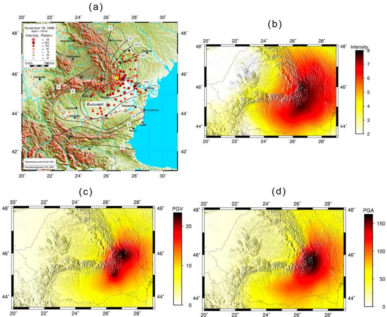
Fig. 6 The intermediate-depth earthquake occurred in the Vrancea seismic zone (event of November 10, 1940,  $M_w$  7.7, depth 140 km). (a) the observed macroseismic map; (b) the modeled distribution of seismic intensity based on FAS-intensity technique; (c) and (d) modeled distribution of Peak Ground Velocity and Acceleration, respectively, using stochastic simulation and site-dependent spectral models.
