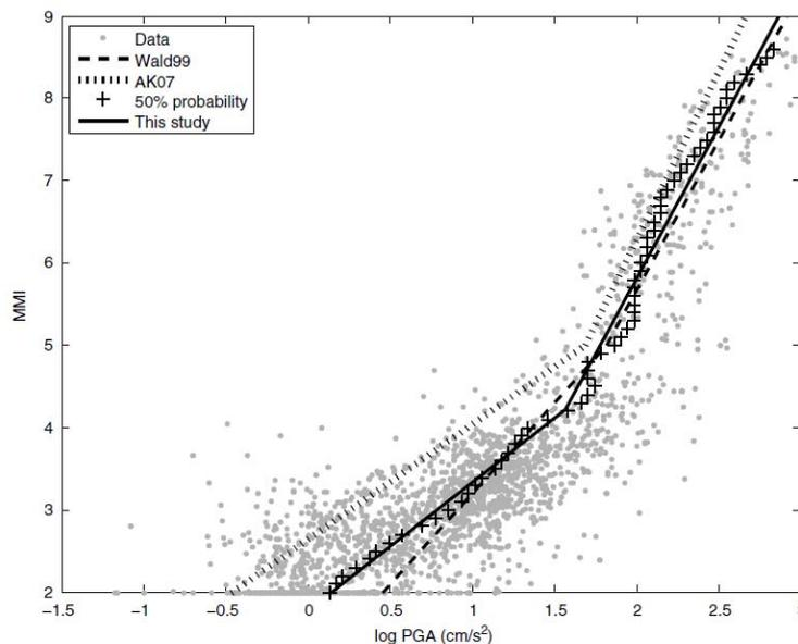
Fig. 1 The PGA versus MMI bilinear total least squares fit (the Figure was taken from Worden et al. 2012, Fig.5)
