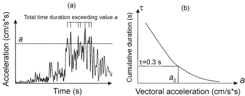
Fig 3. Estimation of JMA instrumental intensity (see text). (a) Calculation of cumulative duration  $\tau$  from vectoral composition of accelerogram. (b) Evaluation of  $a_0$  value used for calculation of the instrumental JMA intensity.
