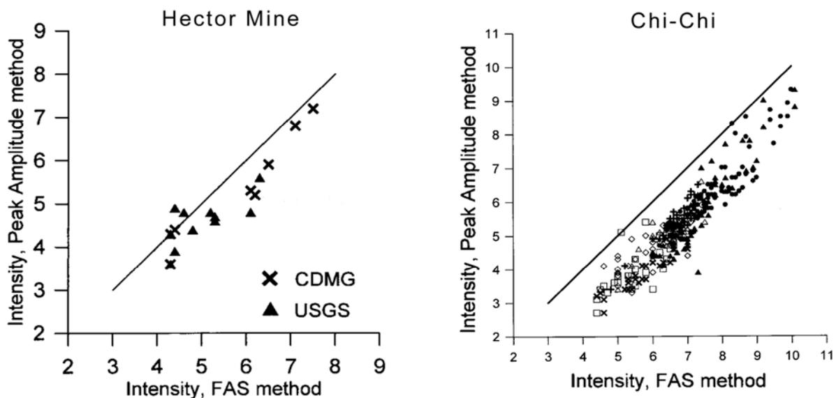
Fig. 7 Comparison between instrumental intensity values calculated from ground-motion records by two methods for the Hector Mine and the Chi-Chi earthquake (Sokolov and Wald 2002). Different symbols denote different arrays of the TSMIP network. Line denotes the direct correspondence between results from the two methods.
