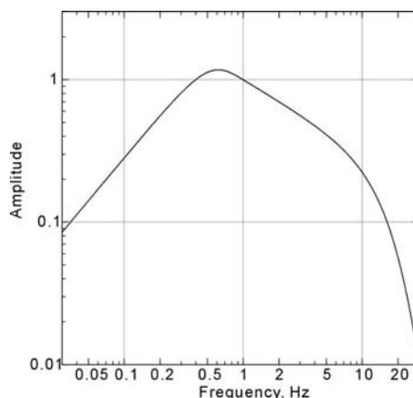
Fig. 2. Response curve of a band-pass filter used for estimating the JMA instrumental intensity (see also <http://www.hp1039.jishin.go.jp/eqchreng/at2-4.htm>).
