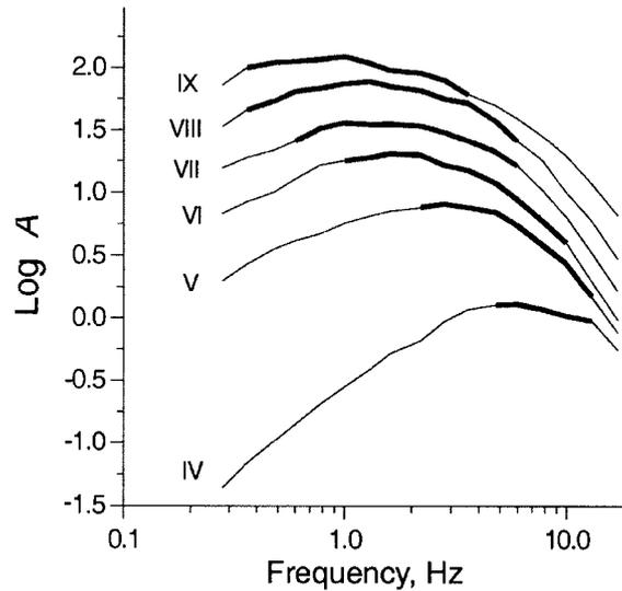
Fig. 4 Mean acceleration spectra ( $A$ , cm/s) for different intensities (IV–IX). Thick lines show spectral amplitudes located within the “representative” frequency ranges (see text)
