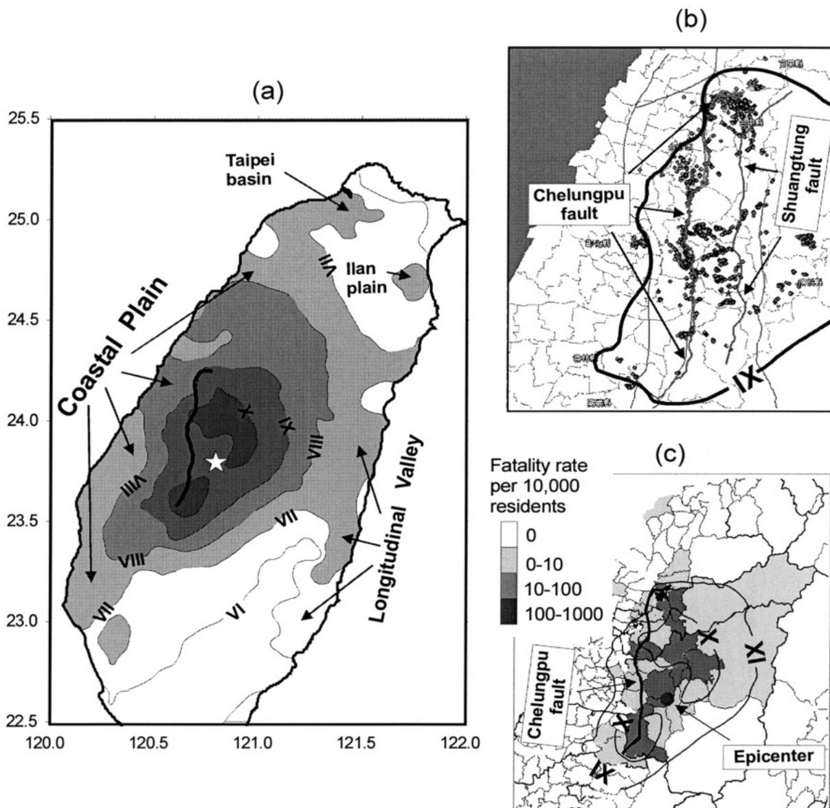
Fig. 8 Instrumental intensity map for the Chi-Chi earthquake according to the FAS method (Sokolov and Wald 2002). (a) Distribution of calculated intensity on the island; (b) epicentral area, with symbols denoting completely collapsed buildings; (c) comparison of instrumental intensity isoseismals and fatality rate (after Y.-B. Tsai, National Central University).
