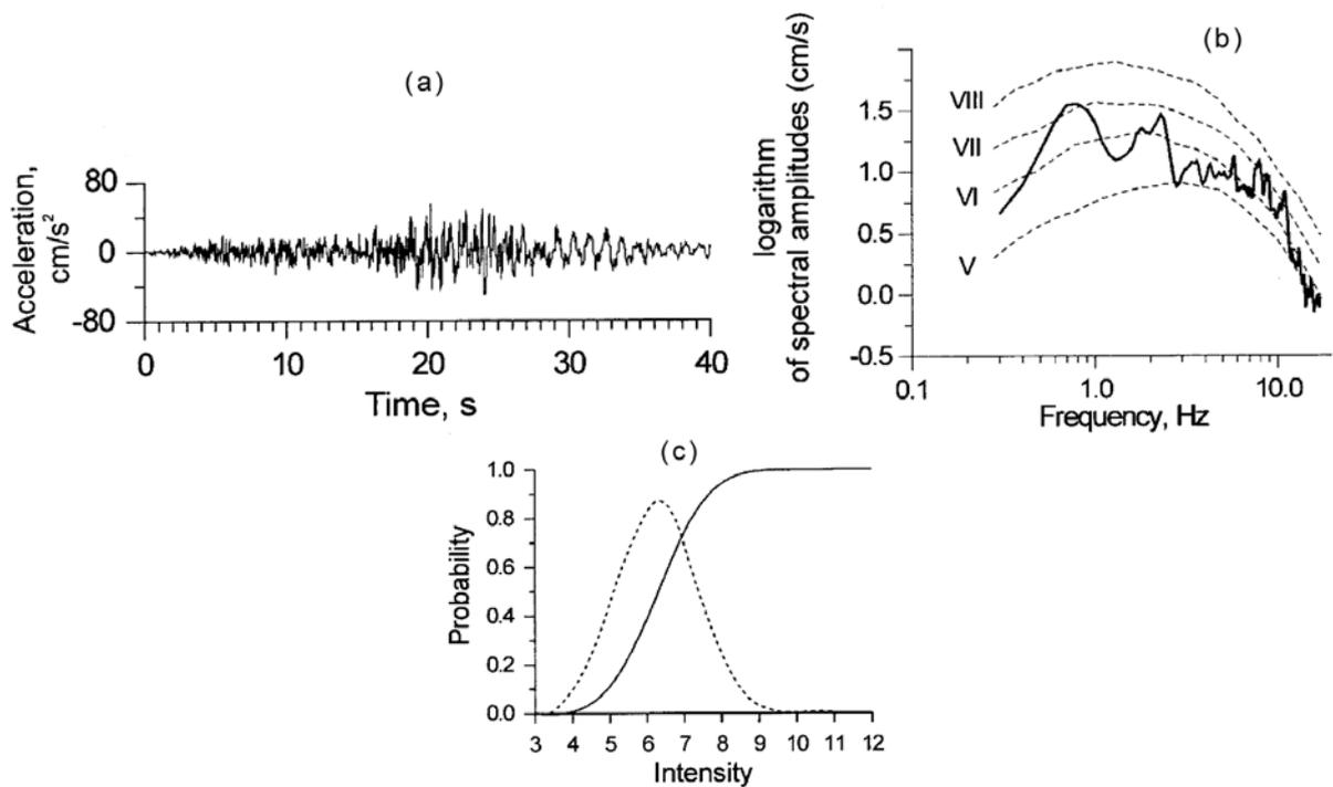
Fig. 5 Seismic-intensity estimation on the basis of FAS (a) acceleration record; (b) comparison of the spectrum of real record (solid line) and the average spectra (dashed lines) for various intensities (MM V–VIII); (c) probability function of intensity not to be exceeded (solid line) and first derivative of the function (dashed line).
