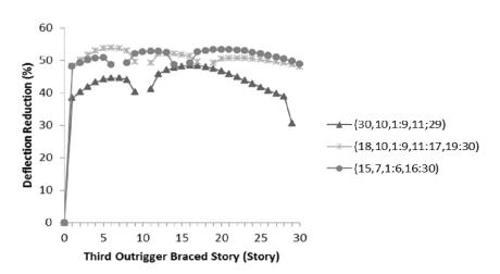
Figure 9. Deflection reduction caused by third outrigger for 30 story model (X-bracing core)
