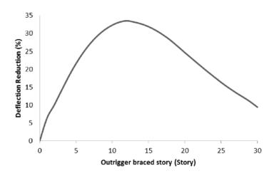
Figure 7. Deflection reduction for 30 story model (X-bracing core)
