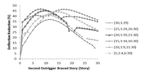
Figure 8. Deflection reduction caused by second outrigger for 30 story model (X-bracing core)
