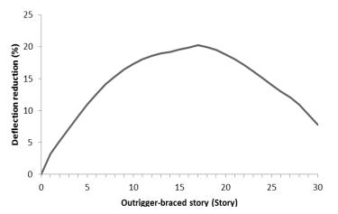
Figure 4. Deflection reduction for 30 story model (V-bracing core)
