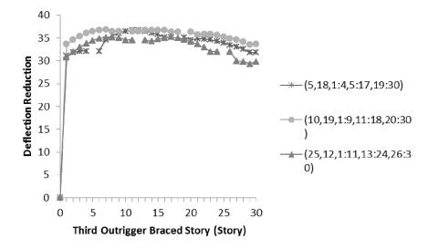
Figure 6. Deflection reduction caused by third outrigger for 30 story model (V-bracing core)
