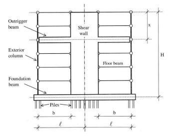
Figure 1. Analytical model of HoenderKramp
