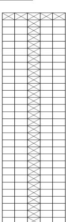
Figure 2. 30 Story V-bracing model
