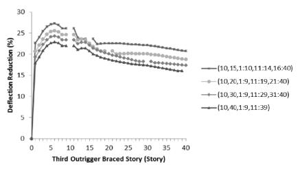
Figure 11. Deflection reduction caused by third outrigger for 40 story model (X-bracing core)
