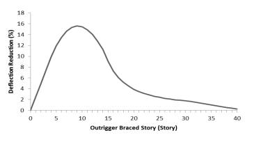
Figure 10. Deflection reduction for 40 story model (X-bracing core)
