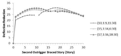
Figure 5. Deflection reduction caused by second outrigger for 30 story model (V-bracing core)
