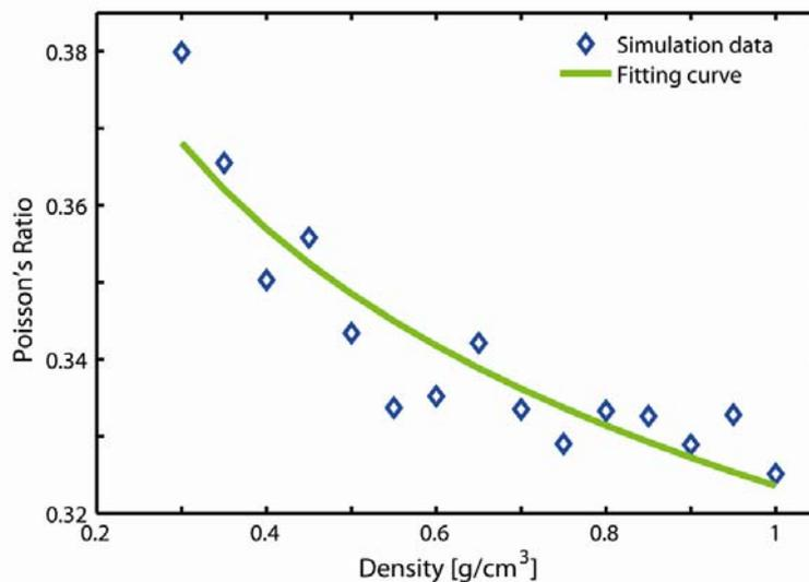
Fig. 3 The relation between Poisson's ratio and the density (The small diamonds refer to the simulation results. The green curve refers to the power-law fitting curve of simulation data.)
