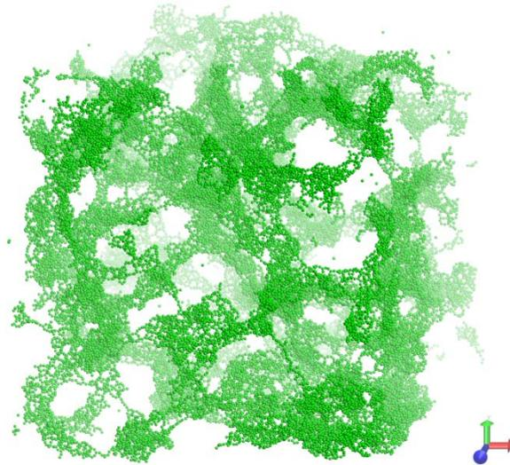
Fig. 1 The model of silica aerogels with the density of  $0.3\text{g/cm}^3$  using molecular dynamics
