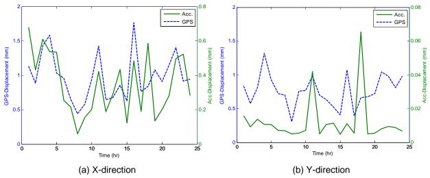
Fig. 5 Dynamic displacements components of GPS and accelerometer in the X-and Y-direction
