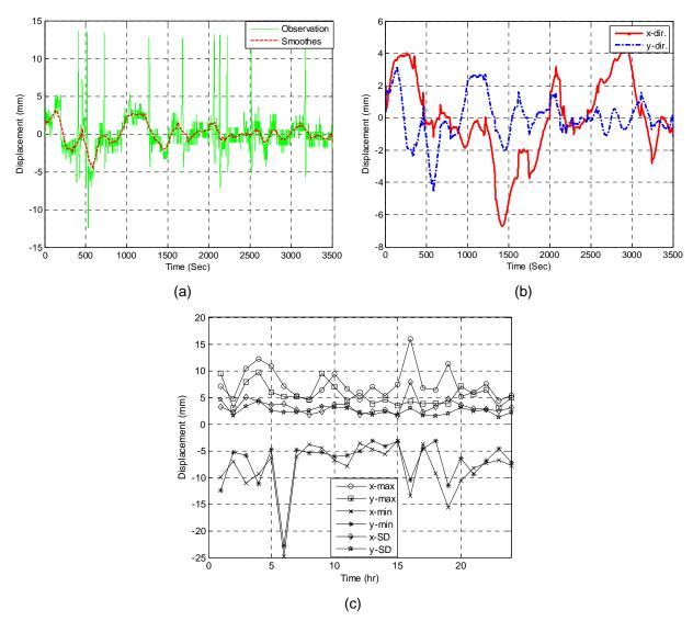
Fig. 4 GPS observations and MA smoothing filter: a) Original and smoothed GPS observations at 23:00; b) GPS smoothed observation of X- and Y-directions at 23:00; c) GPS displacement statistics during the observing day on January 17, 2008
