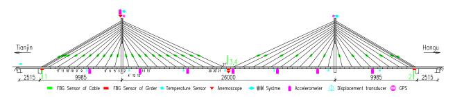
Fig.1 Elevation and SHM system of Yonghe Bridge
