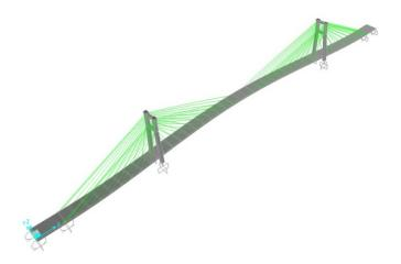
Fig. 3 Yonghe Bridge finite element first mode shape
