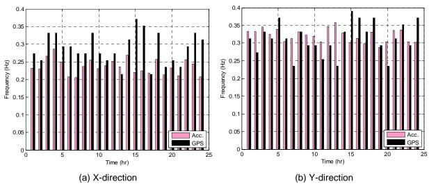
Fig. 7 Fundamental frequencies of the GPS and accelerometer acceleration observations in X- and Y-direction
