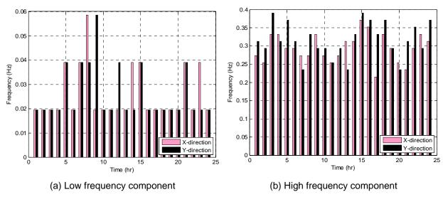
Fig. 6 Fundamental frequency components of the GPS displacement observations in the X- and Y-direction
