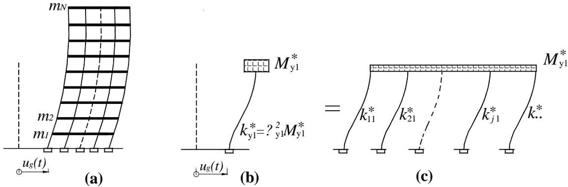
Fig. 2 (a) Typical first mode deformation profile of a multi-story building; (b) the first mode single-story system with the modal stiffness; (c) the contribution of each bent to the modal stiffness
