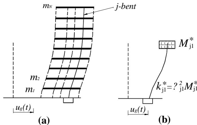
Fig. 3 (a) First mode displacement profile of the multi-story subsystem which has a lateral stiffness depending on the  $j$ -bent; (b) the corresponding SDOF modal system
