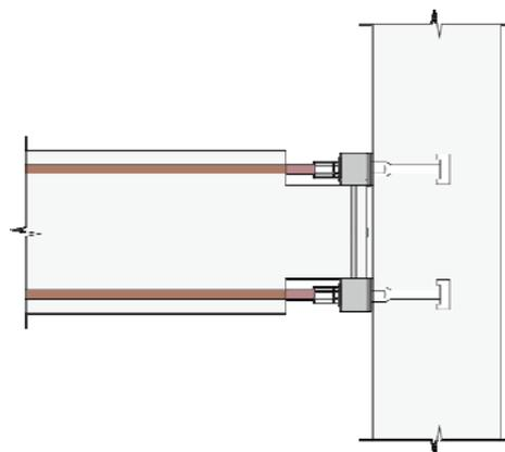
Fig. 1 Pre-tension bolting connection concept
