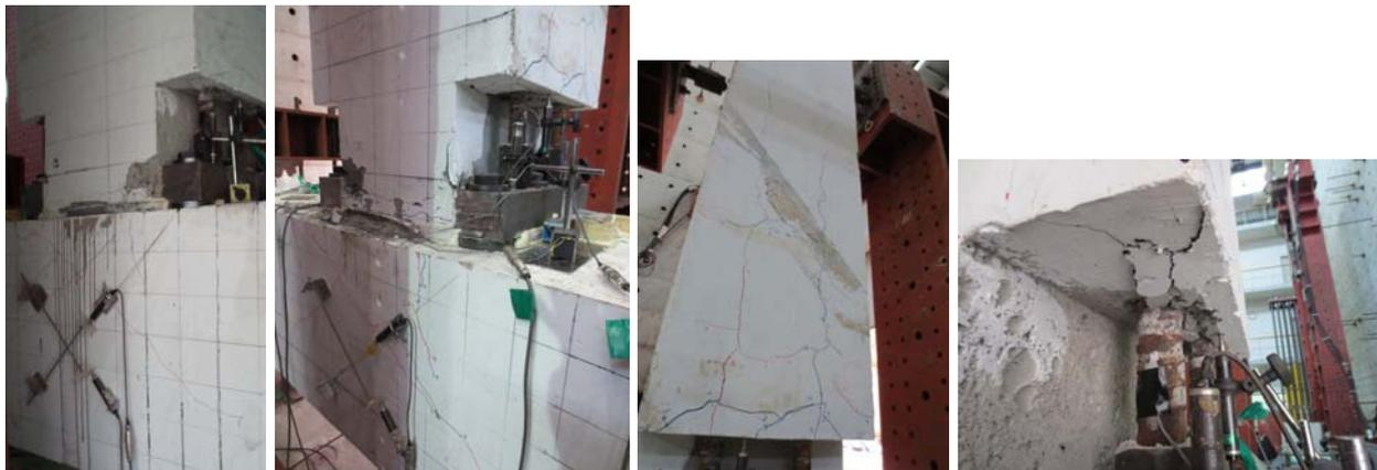
Fig. 10 Observations of PC2-T at 4% drift ratio
