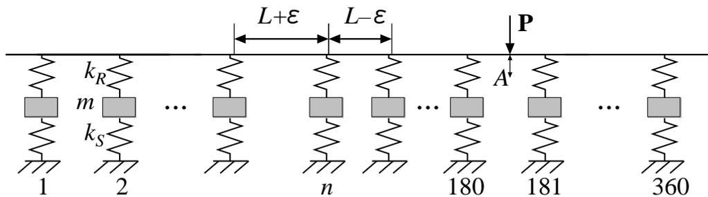
Fig. 3 Track model that  $n$ th sleeper location is shifted
