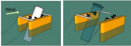
Figure 4: Flexible supporting system of the turbine shaft
