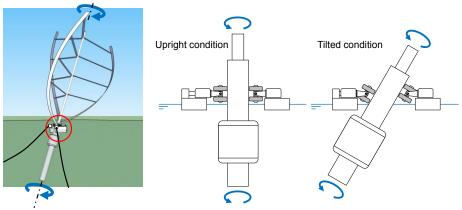
Figure 2: Floating Axis Wind Turbine concept; (a) overall view and (b) flexible turbine support
