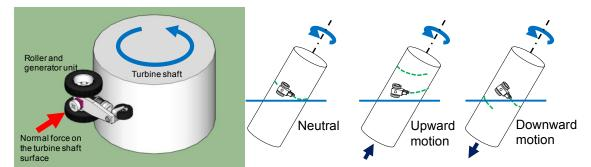
Figure 3: Flexible supporting system of the turbine shaft; (a) roller and generator unit and (b) the treatment of relative heave motion
