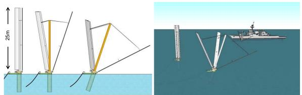
Figure 5: Mobile FAWT concept (Foldable blade, mobile floating wind turbine)
