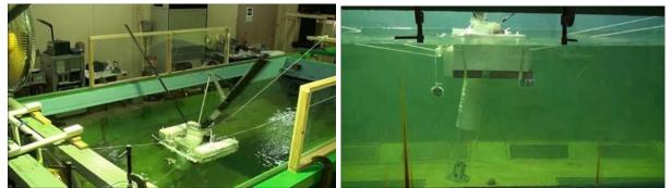
Figure 6: Snap shots of preliminary experiments; (left) rotating wind turbine part and (right) side view of the submerged part
