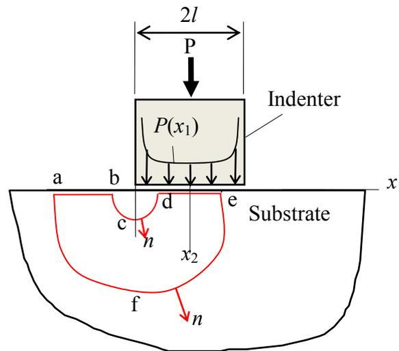
Fig.2 Integration path for homogenous substrate.
