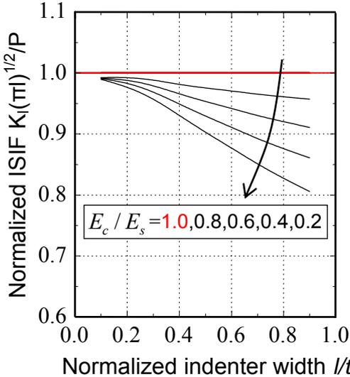
Fig.6 Normalized stress intensity factors for different parameters
