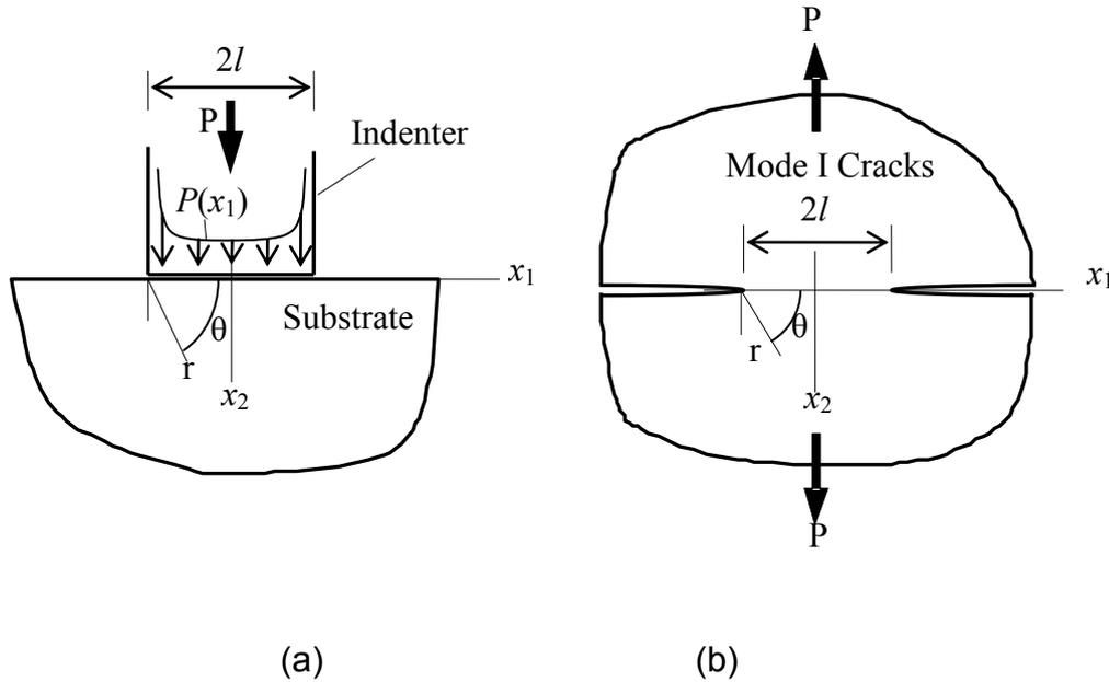
Fig.1 A schematic representation of the indentation. (a) Contact by a rigid flat-end indenter. (b) Related Mode I crack.
