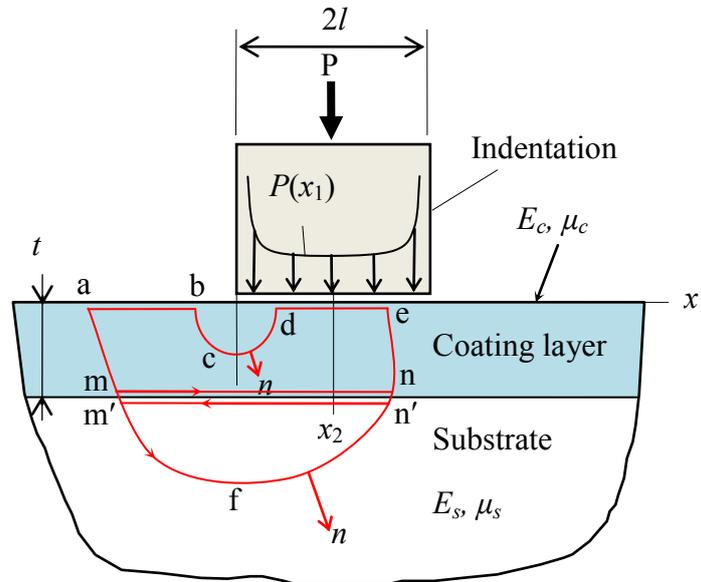
Fig.3 Indentation path for the layered substrate
