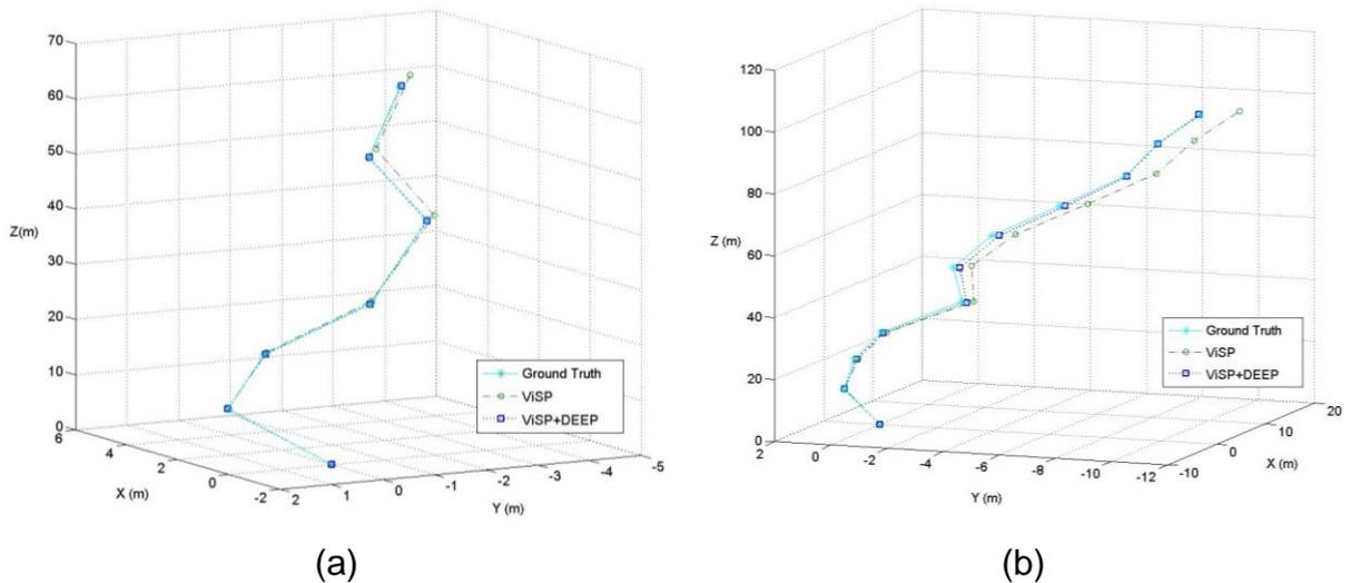
Fig. 2 Simulation results with six and ten modules. Solid line with asterisk: ground truth. Dot dashed line with circle: estimated displacement from ViSP. Dotted line with rectangle: updated displacement by using DEEP method
