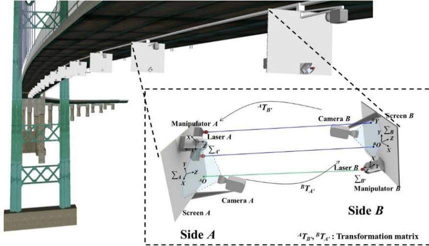
Fig. 1 Application of multiple visually servoed paired structured light system to civil structures. Details of ViSP can be found inside a dashed line box.
